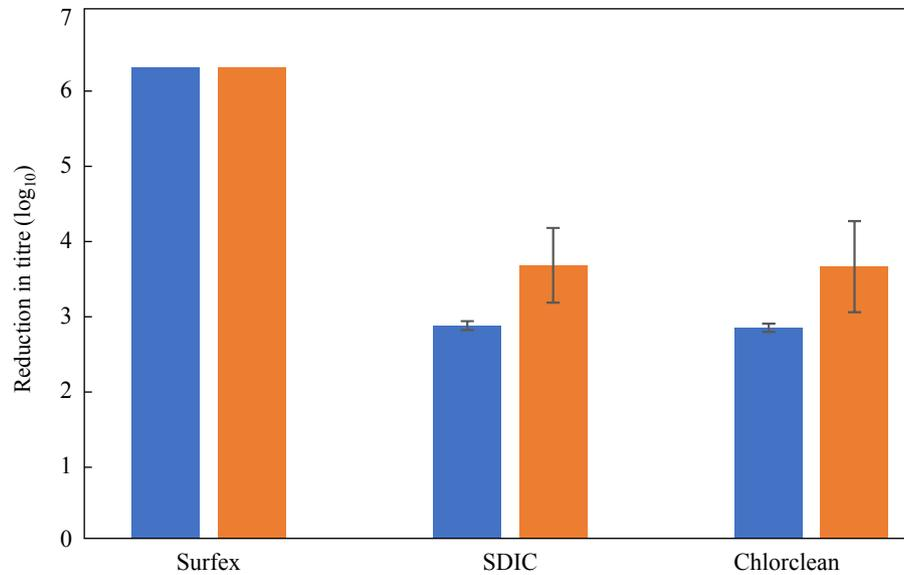
**Figure 4.** Reduction in dry-surface biofilm titre ( $\log_{10}$ ), in the absence of biological soil, obtained with (orange bars) and without (blue bars) prior biofilm contact with detergent (Speedy Clean for 30 s) followed by Surfex, sodium dichloroisocyanurate (SDIC) and Chlorclean disinfection for a contact time of 5 min.
