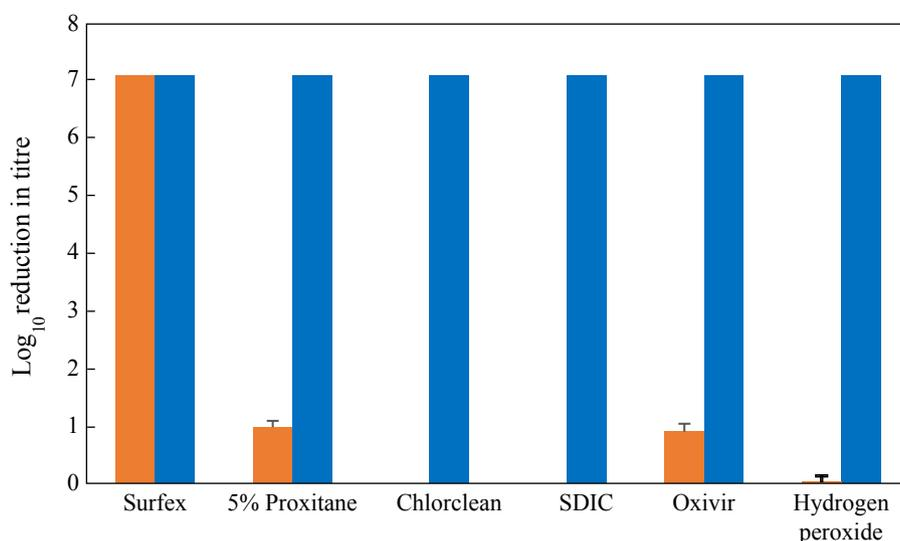
**Figure 2.**  $\log_{10}$  reduction in planktonic *Staphylococcus aureus* titre following a 5-min contact with disinfectants containing peracetic acid and hydrogen peroxide (Surfex, Proxitane), chlorine [Chlorclean, sodium dichloroisocyanurate (SDIC)] and hydrogen peroxide (Oxivir, hydrogen peroxide) as active ingredients. Disinfectant efficacy was determined in hard water with (orange bars) and without (blue bars) added biological soil.
