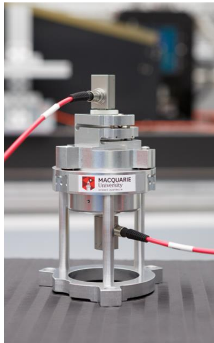
Figure 2: Left: CAD rendering of the science etalon mounting mechanics. The assembly is designed to be mounted inside a standard ISO-K 160 tube (only the lower end flange is shown). Components in green are made from G10 for thermal decoupling. Right: photo of etalon mechanical assembly, which was used for initial alignment of the Veloce spectrograph, part of which can be seen in the background.
