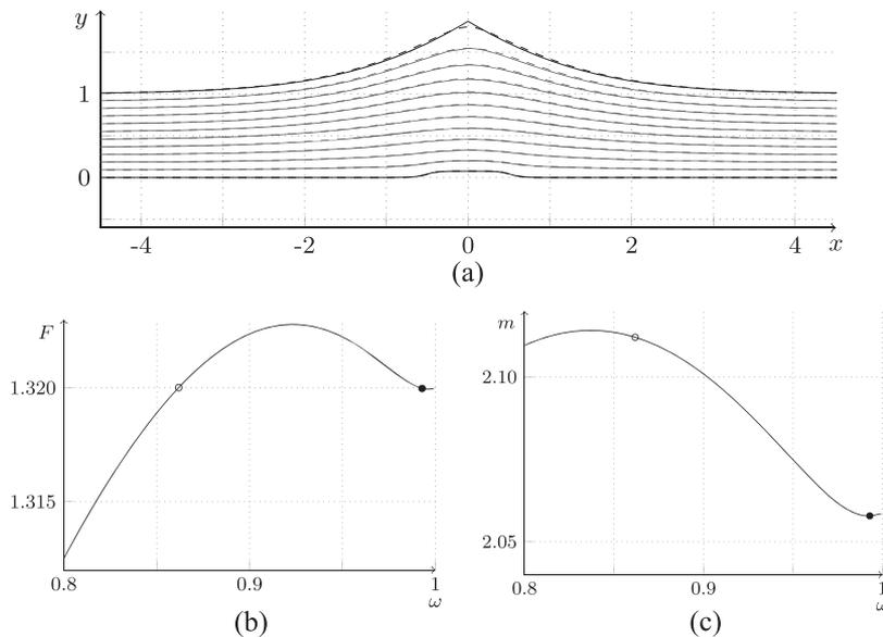
FIG. 8. Analysis of almost-highest type-II solutions with  $A = 0.079$ . (a) Streamlines for two almost-highest type-II solutions with  $F = 1.32$ . Broken curves,  $\omega = 0.862$ ; solid curves,  $\omega = 0.993$ . [(b) and (c)] Plots of the Froude number  $F$  and wave mass  $m$  versus  $\omega$ . The markers indicate the location of the solutions shown in (a).
