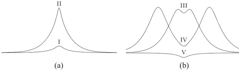
FIG. 1. Sketch of the five basic types of solutions for localized forcing due to either a distribution of pressure on the free surface or a topographical disturbance on the bottom of the channel,  $F > 1$ . (a) Forcing with  $A > 0$  and (b)  $A < 0$ .
