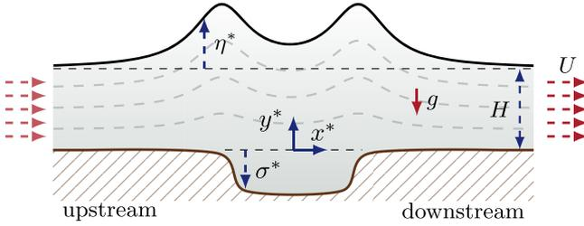
FIG. 2. Schematic of the steady flow problem. The free surface is denoted by  $y^* = H + \eta^*$ . The topography,  $y = \sigma^*$ , is stationary with respect to the wave crest(s).
