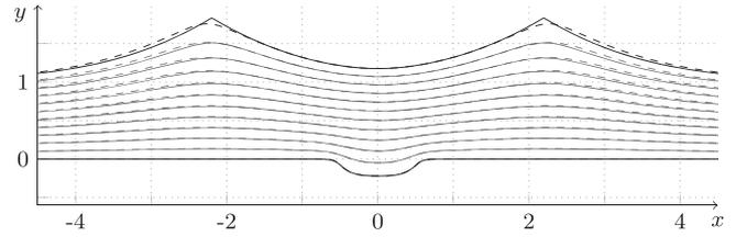
FIG. 7. Streamlines for two almost-highest type-IV solutions with  $F = 1.2906$  and  $A = -0.196$ . Broken curves,  $\omega = 0.813$ ; solid curves,  $\omega = 0.990$ .
