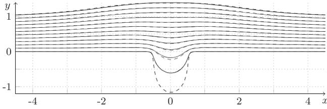
FIG. 5. Streamlines for two type-II solutions with  $F = 1.16$ . Solid curves,  $A = -0.5$ ; broken curves,  $A = -1.0$ .
