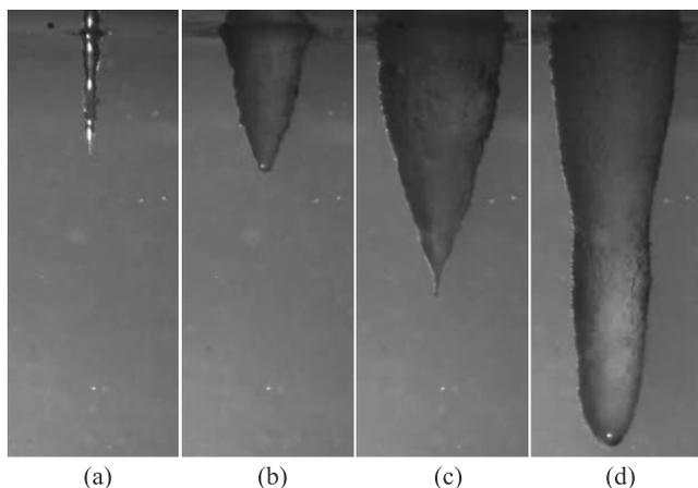
Fig. 5. Laser beam interaction with a gelatin sample.
