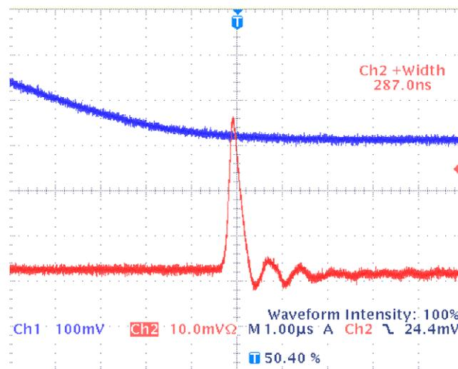
Fig. 4. Oscilloscope pictures of the shortest Q-switch pulse generated by the Er:YAG laser. Lower trace – laser pulse, upper trace – current applied to the pump lamp.
