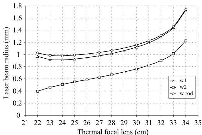
Fig. 2. Calculated dependence of fundamental mode radius on M1 and M2 mirrors and in a laser rod (for the laser presented in Fig. 1) vs. focal length of a thin lens representing a thermal lens of an active laser rod. w1, w2 – radius of a laser beam located on M1 and M2 mirrors, respectively; w rod – radius of a laser beam at the centre of a laser rod.
