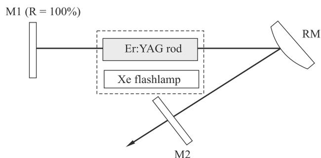
Fig. 1. Q-switched Er:YAG laser set-up with thermal lensing compensation.
