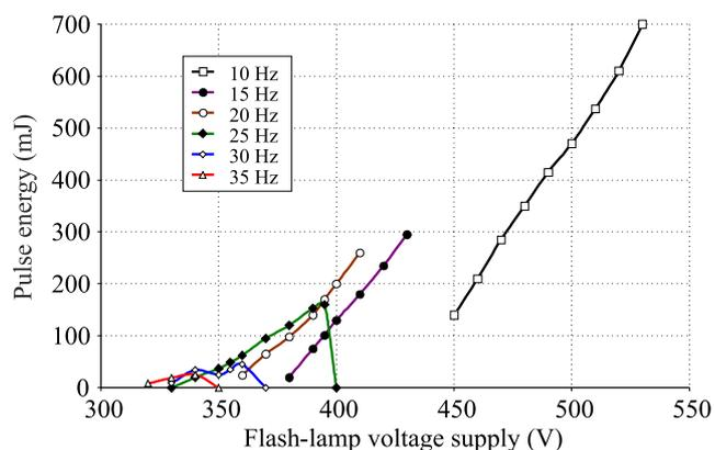
Fig. 3. Output energy of free-running Er:YAG laser vs. flash-lamp supply voltage for repetition rates of 10, 15, 20, 25, 30, and 35 Hz. Pump pulse duration – 300  $\mu$ s.
