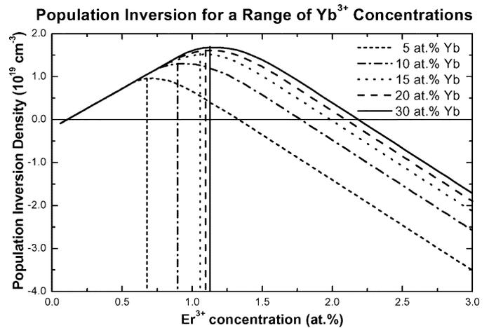
Fig. 6. Population inversion densities ( $N_{\text{upper}} - N_{\text{lower}}$ ) in Er<sup>3+</sup> for a range of Yb<sup>3+</sup> concentrations. The optimum Er<sup>3+</sup> concentration (i.e. at the maximum inversion) is marked.
