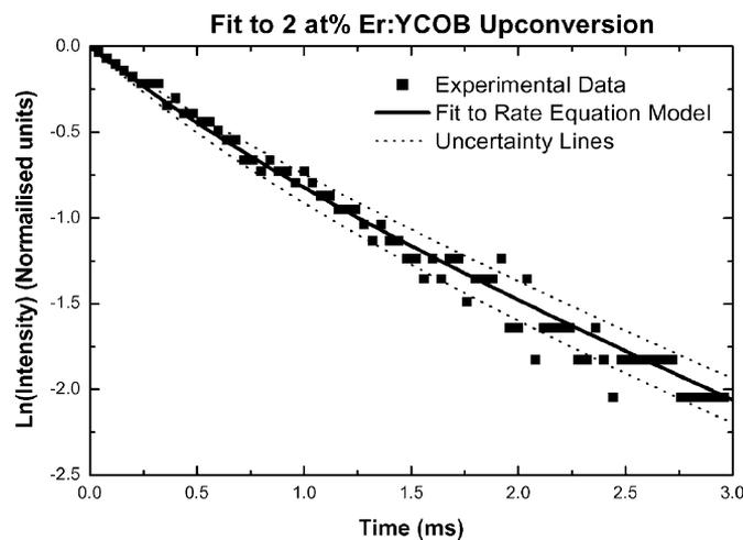
Fig. 2. Fit of the <sup>4</sup>I<sub>13/2</sub> population decay in 2 at.% Er:YCOB to (A4) with upconversion parameters of  $W_{UC} = 1.30 \times 10^{-17} \text{ s}^{-1}$ . The dotted lines indicate  $\pm 0.4 \times 10^{-17} \text{ s}^{-1}$  uncertainty margins.
