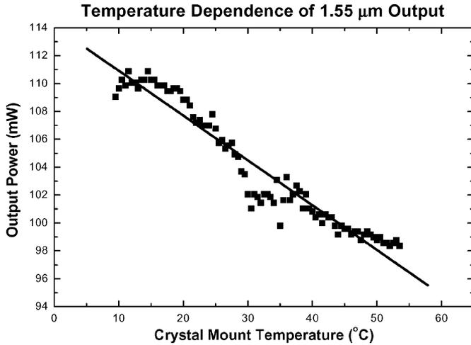
Fig. 10. Temperature dependence of laser output (1% 200 mm OC). The degradation of output power with temperature is  $-0.3 \text{ mW}/^\circ\text{C}$ .
