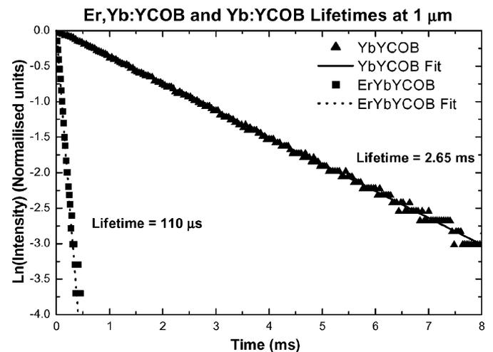
Fig. 4. Comparison between the lifetimes of the <sup>2</sup>F<sub>5/2</sub> manifold of the Yb<sup>3+</sup> sensitizer ions in the singly doped Yb:YCOB, and the codoped Er,Yb:YCOB.
