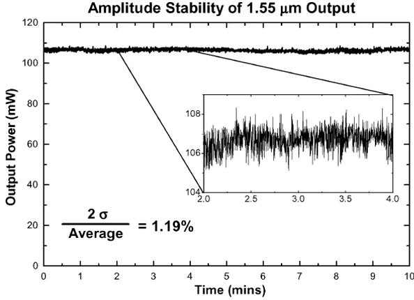
Fig. 9. Amplitude stability of 1.55- $\mu\text{m}$  laser output at maximum power (1% 200 mm OC).
