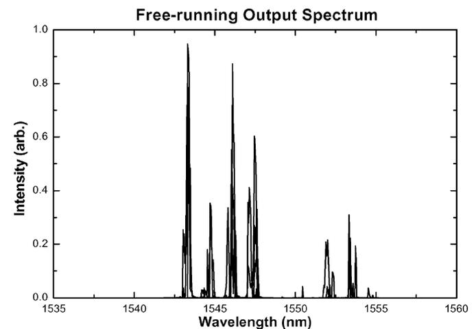
Fig. 8. Free-running output spectrum of the Er,Yb:YCOB laser in the flat-flat cavity configuration. Spectrum is the accumulation of seven individual wavelength scans.
