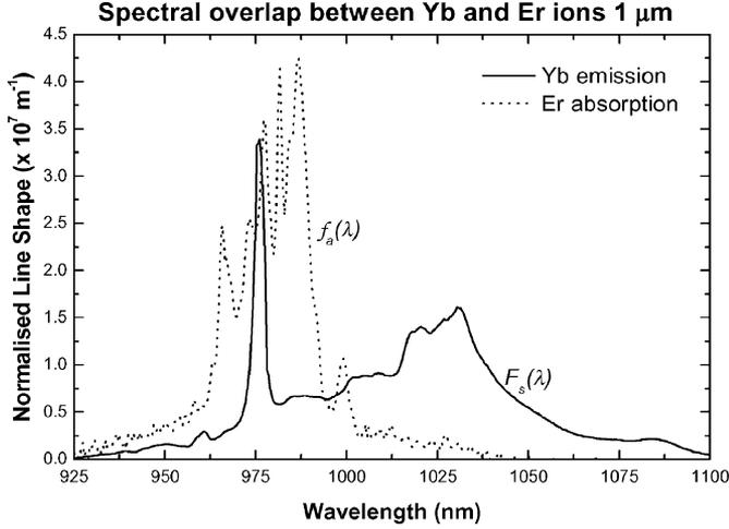
Fig. 1. Spectral overlap between the emission of the  $\text{Yb}^{3+}$  sensitizer ions,  $F_s(\lambda)$ , and the absorption of the  $\text{Er}^{3+}$  activator ions,  $f_a(\lambda)$ .
