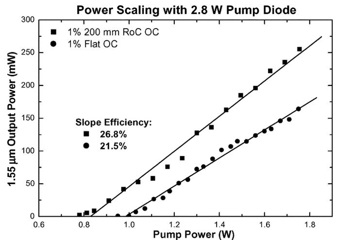
Fig. 7. Er,Yb:YCOB laser output using the 2.8 W fiber coupled diode pump laser. The maximum output was  $\sim 250 \text{ mW}$  of CW radiation.
