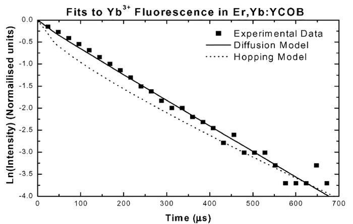
Fig. 3. Fits of the fluorescence decay of the Yb<sup>3+</sup> <sup>2</sup>F<sub>5/2</sub> manifold in the Er,Yb:YCOB crystal to the characteristic decay of the diffusion and hopping models.
