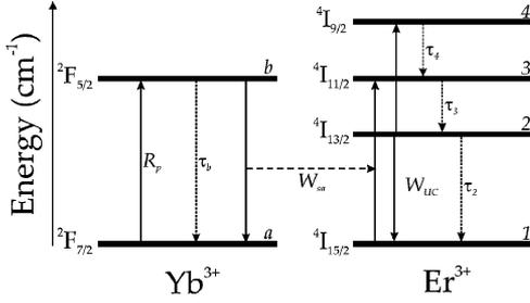
Fig. 5. Level assignment diagram and relevant processes for rate equation analysis of the Er,Yb:YCOB laser material.
