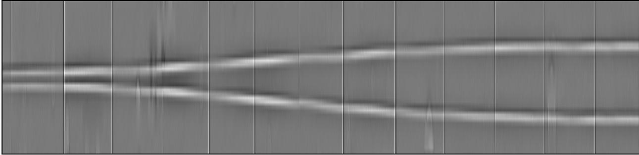
Figure 3. Transmission phase contrast micrographs stitched together showing half of a 2x2 evanescent coupler fabricated in Yb-doped borosilicate glass using the femtosecond laser direct-write technique. Image not to scale.
