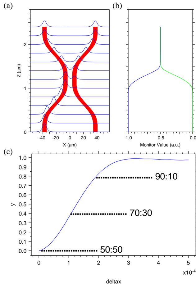
Figure 1. (a) Beam propagation simulation (RSoft) of a 2x2 coupler in Yb-doped borosilicate glass. (b) Monitored 800 nm light guided in each coupler arm along the device. (c) Difference in splitting ratio at the coupler's exit when the device's refractive index (deltax) is varied where 976 nm light propagates.
