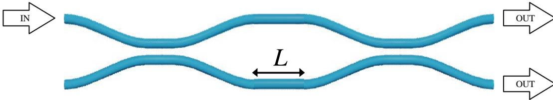
Figure 2. Schematic of a Mach-Zehnder interferometer incorporating two 50:50 splitters separated by a linear region of length  $L$ .
