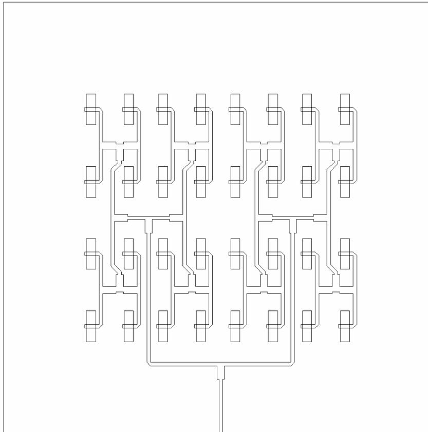
Fig. 2. Stripline feed network for the dual resonator 1-D EBG antenna consisting of a 4x8 slot array. Slots are superimposed on the stripline network to show relative position.
