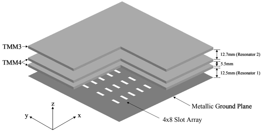
Fig. 1. Dual resonator 1-D EBG antenna with slot array feed realized using Rogers TMM dielectric sheets with dimensions 152mm x 152mm x 3.18mm. One quarter of the TMM sheets has been cut away to show the slot array more clearly.
