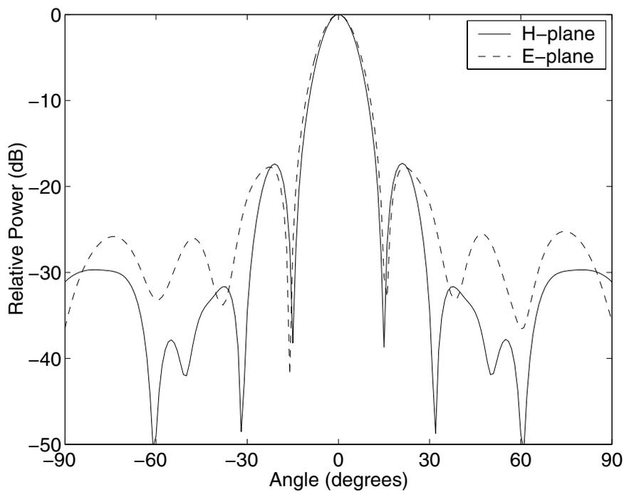
Fig. 3. Computed *H*- and *E*-plane radiation patterns at 12.1GHz.
