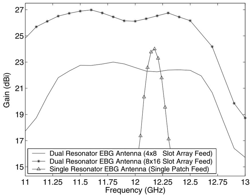
Fig. 4. Theoretical gain for dual resonator 1-D EBG antennas (4x8 slot array feed and 8x16 slot array feed) compared with a classical single resonator EBG antenna.
