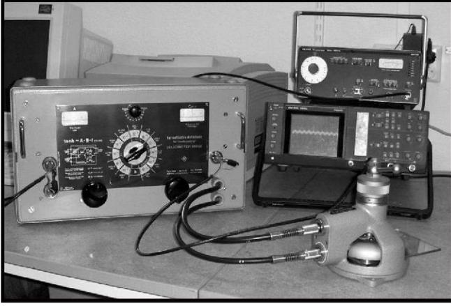
Fig. 1. Photograph showing the setup of the parallel plate guard ring capacitor measurement method
