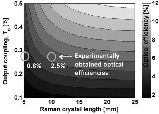
Fig. 8. Modeled efficiency of the Raman laser as a function of the Raman crystal length ( $l_r$ ) and output coupling transmission for Stokes ( $T_s$ ) at an absorbed pump power ( $P_p$ ) of 33 W.
