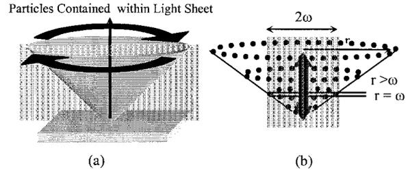
Fig. 2. (a) Three-dimensional rotational analysis of the droplets contained within each image (front view). (b) Adjustment for the finite width of the light sheet (side view).
