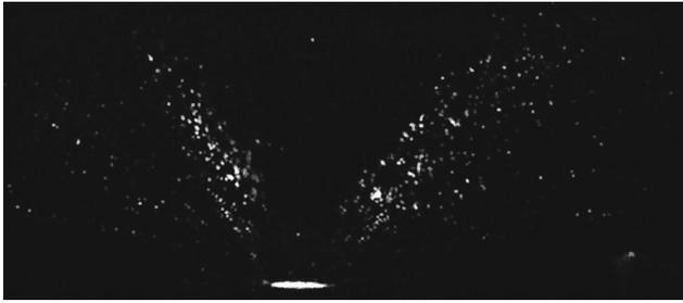
Fig. 1. Typical gray-scale image obtained during ablation with a visible nanosecond laser pulse.
