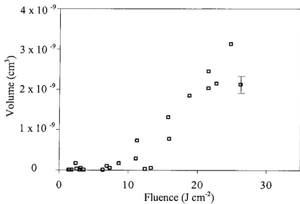
Fig. 7. Volume of material ejected as a result of ablation with increasing fluence (spot radius,  $\sim 37 \mu\text{m}$ ).
