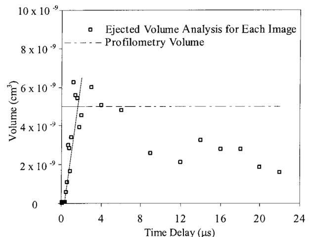
Fig. 6. Volume of melt ejecta contained within images taken at increasing time delays after ablation with a single  $\sim 40\text{-J cm}^{-2}$ , 30-ns pulse.
