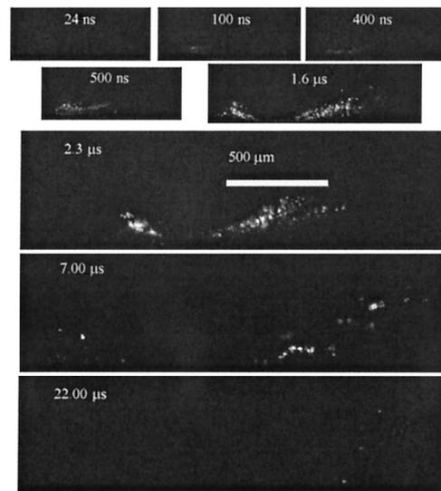
Fig. 5. Images showing the temporal evolution of ejected material as a result of a single  $\sim 40\text{-J cm}^{-2}$ , 30-ns pulse.
