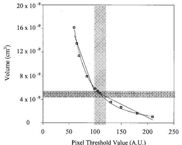
Fig. 3. Volumes obtained from a single image as a function of pixel threshold. (Shaded regions demarcate boundaries of reasonable pixel values as determined by errors in the  $x$  and  $y$  axes.)
