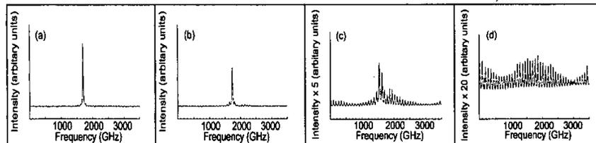
Fig. 2. The optical frequency spectrum from the TSL with  $I_L = 64.9$  mA,  $I_A = 2.0$  mA,  $f_M = 960$  MHz and variable modulation power: (a) 0 dBm, (b) 2 dBm, (c) 7.6 dBm and (d) 15 dBm. The frequency scale is relative and centred about the laser wavelength of  $\sim 850$  nm.
