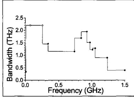
Fig. 3: Bandwidth of the optical frequency spectrum as a function of modulation frequency for  $I_L = 69.5$  mA,  $I_A = 2.0$  mA and modulation power = 7 dBm. Closed circles correspond to a bandwidth below the FSR of the FP interferometer, open circles indicate the bandwidth exceeded that of the FSR.
