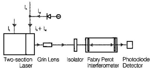
Fig.1: A schematic of the two-section laser showing injection currents to the two-sections and the diagnostics for monitoring the optical frequency spectrum.
