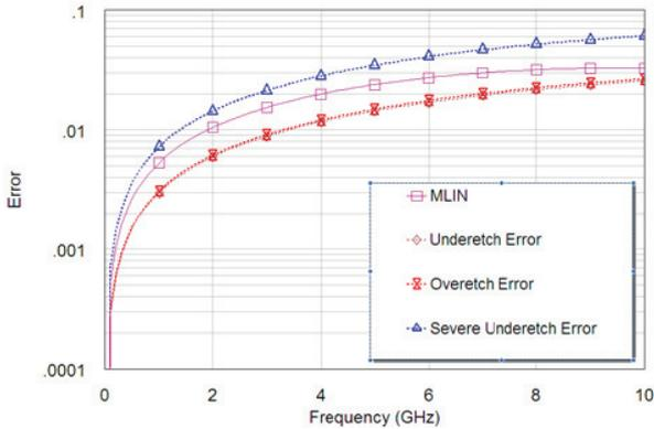
Figure 1 – MLIN, -1 mil overetch, +1 mil underetch, and +2 mil severe underetch error relative to nominal W=20 mil line
