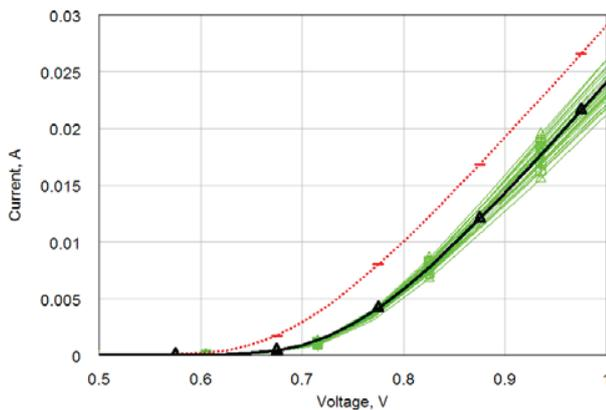
Figure 3 – I-V data for MMIC HBT diode showing nominal process model (dotted line), extracted model for average measured data (thick solid line) and measured data for 30 diodes (thin solid lines).
