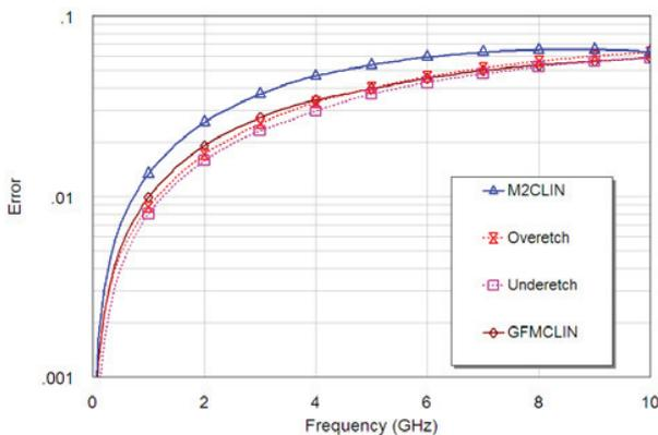
Figure 2 – M2CLIN, Overetch, Underetch, and GFMCLIN error relative to nominal  $W=6$   $S=9$  coupled microstrip
