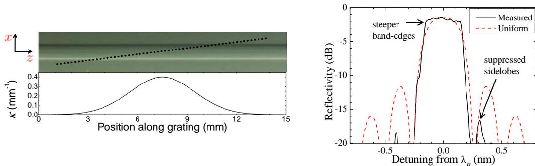
Fig. 2 (Left) Illustration of the Gaussian apodization technique. (Right) Reflection spectrum of a sinc-apodized FBG (black solid) compared to a simulation of a uniform FBG with equivalent strength and bandwidth (red dashed).
