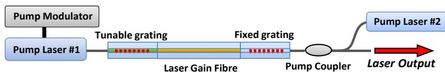
Fig. 1 Layout of the Q-switched fibre laser cavity.
