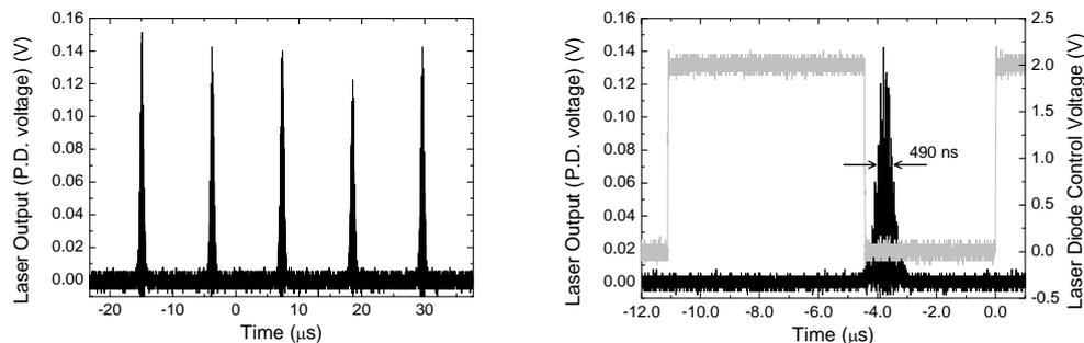
Fig. 3 Output pulses from the Q-switched fibre laser at 90 kHz. The diode control pulse for driving the Q-switch is shown in grey (right).
