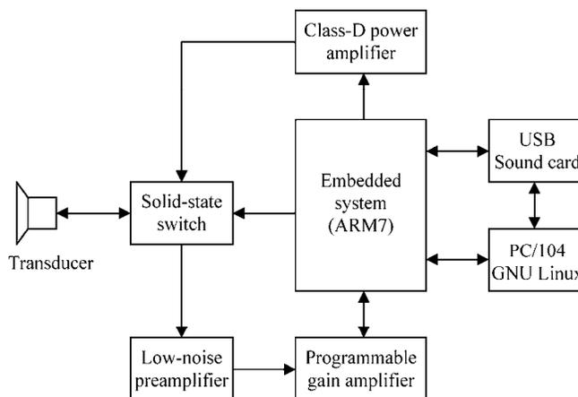
Figure 3 High level overview of Snodar's electrical system<sup>11</sup>. A PC/104 computer running Linux performs all the signal processing and control tasks in real time. A USB sound card provides 24-bit analogue signal acquisition at a sampling frequency of 96kHz. The ARM7TDMI embedded system provides system control and data acquisition.
