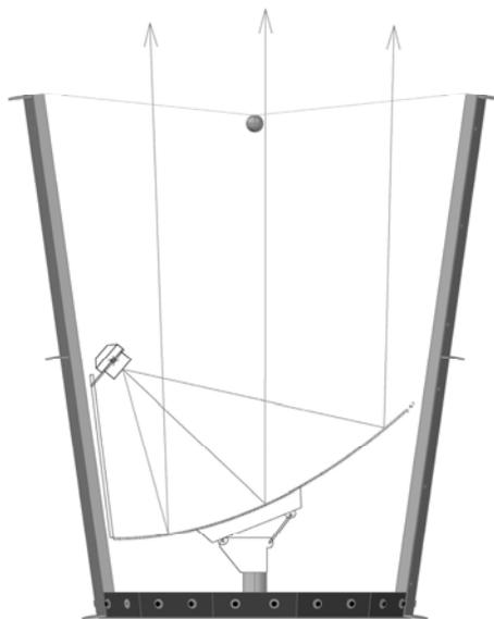
Figure 2 Cross section of Snodar's antenna<sup>10</sup>: the acoustic transducer is near the focal point of a 0.9 m f/0.6 off-axis parabolic reflector housed in a 1.6 m tall sound cone. The calibration sphere is suspended in the middle of the sound cone's aperture.
