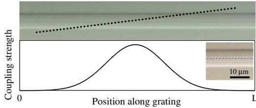
Fig. 1. (Color online) Illustration of the Gaussian apodization technique: a linear translation of focus across the core produces a Gaussian apodization profile. Inset, micrograph of a PbP FBG in SMF-28e fiber.
