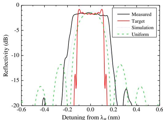
Fig. 4. (Color online) Measured reflection spectrum of the sinc-apodized grating (solid black curve), target spectrum based on  $\kappa(z)$  shown in Fig. 3 (solid red curve), simulated spectrum of the fabricated grating (dotted blue curve), and modeled spectrum of a uniform FBG (dashed green curve).
