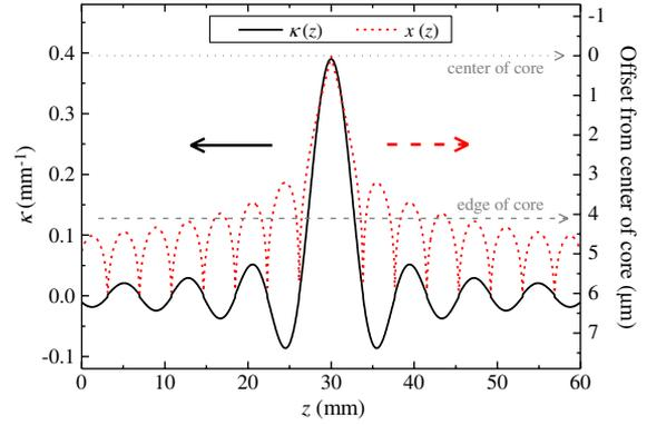
Fig. 3. (Color online) Coupling amplitude ( $\kappa$ ) profile (black curve) and translation function (red curve) for a sinc-apodized PbP grating.
