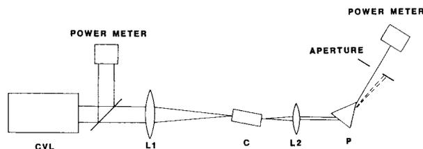
Fig. 1. Schematic diagram of experimental arrangement used for sum frequency generation.
