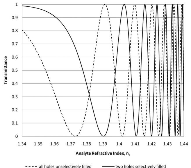
Fig. 3. Plot of transmittance of a 2 mm length of the dual-core sensing fiber for vertically polarized input as a function of analyte refractive index for (i) all holes nonselectively filled with analyte (dotted curve) and (ii) only the two holes between the cores selectively filled with analyte (solid curve).
