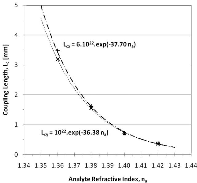
Fig. 2. Plot of coupling length versus analyte refractive index when all holes in the microstructure are filled with analyte: +, input polarization vertical; ×, input polarization horizontal.
