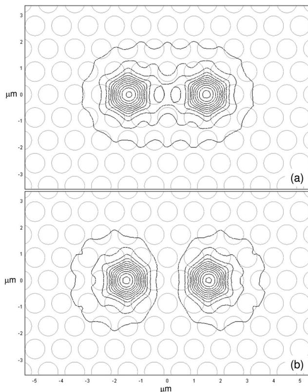
Fig. 1. Plot of intensity distribution of (a) even and (b) odd supermodes at  $\lambda=633$  nm in a dual-core microstructured fiber with hole diameter  $d=0.750$   $\mu\text{m}$  and hole pitch  $\Lambda=1$   $\mu\text{m}$ . The refractive index of the host is  $n_{\text{host}}=1.45$ , and all holes are assumed to be filled with an analyte with refractive index  $n_a=1.42$ . The horizontal and vertical scales are in micrometers.
