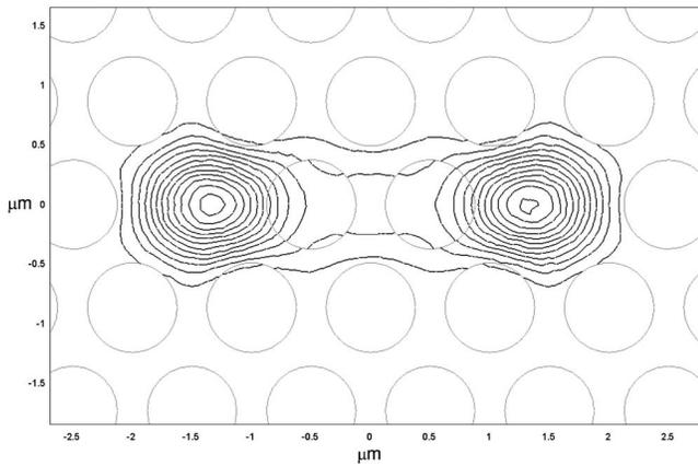
Fig. 4. Plot of the intensity distribution of the even supermode in the same structure as shown in Fig. 1, except for selective filling of only the two holes between the two cores with analyte (all other holes are assumed air filled). The horizontal and vertical scales are in micrometers.
