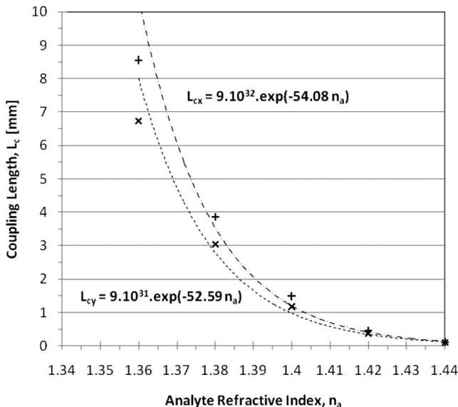
Fig. 5. Plot of coupling length versus analyte refractive index in the selectively filled microstructure. +, input polarization vertical; ×, input polarization horizontal.
