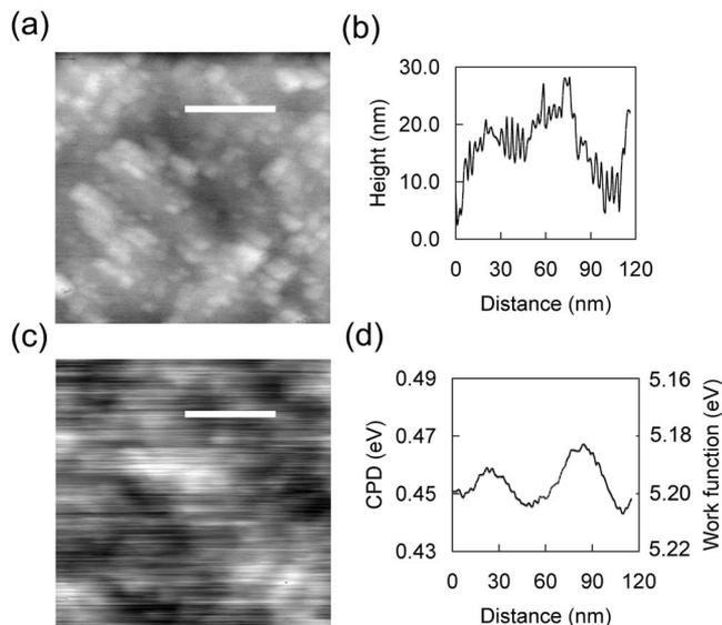
FIG. 1. Noncontact AFM (a) and Kelvin-probe (c) images obtained for the same area of the polycrystalline sample (sample I), immediately after insertion into UHV; the scan size is  $350 \text{ nm} \times 350 \text{ nm}$  in each case. [(b) and (d)] show scans of surface topography and CPD along the lines indicated in the corresponding images.
