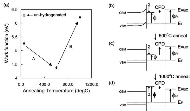
FIG. 2. (a) Measured work function of virgin and annealed hydrogenated surfaces (●) and unhydrogenated surface (○) for sample I. Anneal A: 600 °C; anneal B: 1000 °C. [(b)–(d)] Schematic representation (not to scale) of the band-edge diagram at the hydrogenated diamond surface, relative to the probe: (b) virgin H-terminated film exposed to atmosphere; (c) H-terminated film following 600 °C anneal; (d) H-desorbed film following 1000 °C anneal.
