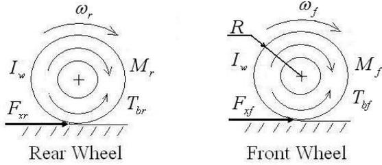
Fig. 3. Torques acting on front and rear tires
