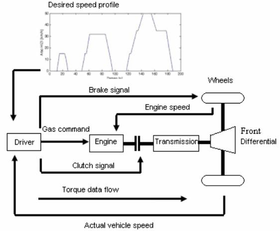
Fig. 1. Forward data flow computation technique and typical urban driving speed profile
