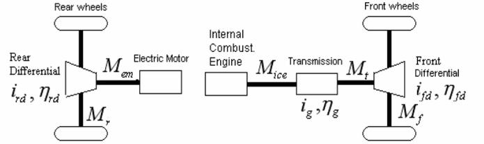
Fig. 5. Driveline components
