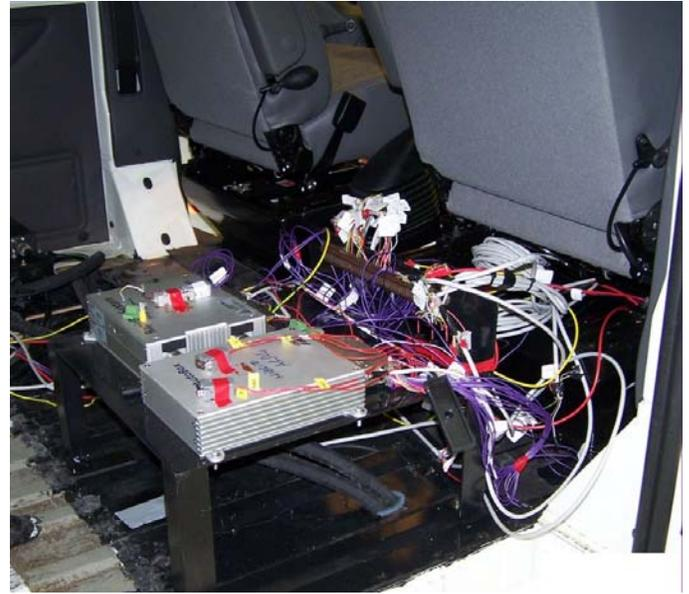
Fig. 12. HEV controller hardware connections in the experimental vehicle
