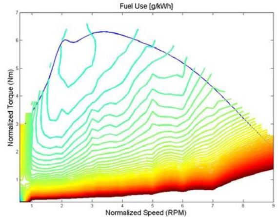
Fig. 6. Engine Fuel Consumption Map
