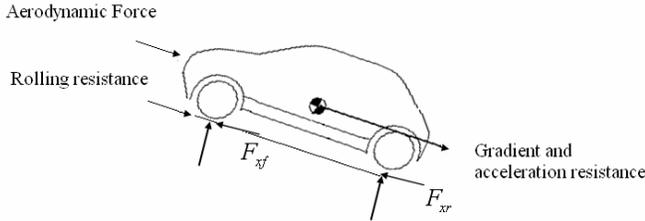
Fig. 4. Longitudinal forces acting on the vehicle
