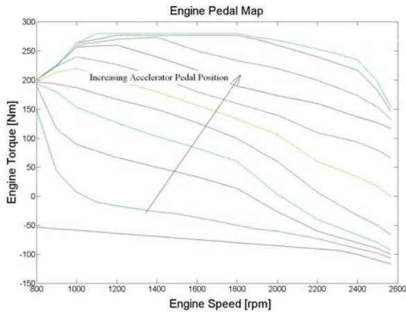
Fig. 9. Engine pedal map versus engine speed and engine torque characteristics
