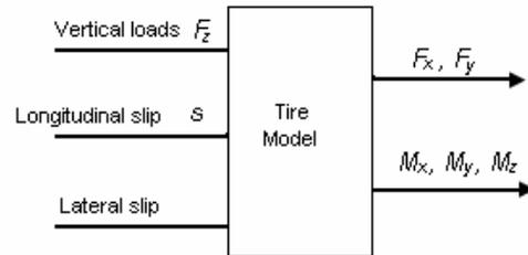
Fig.2. Tire model input and outputs
