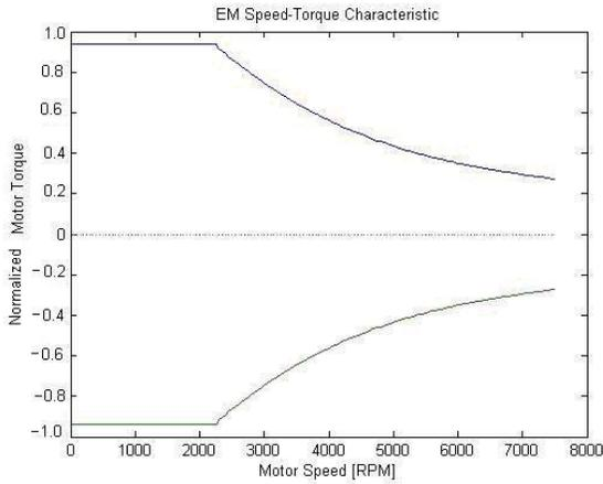
Fig. 7. EM Torque – Rotor Speed characteristics
