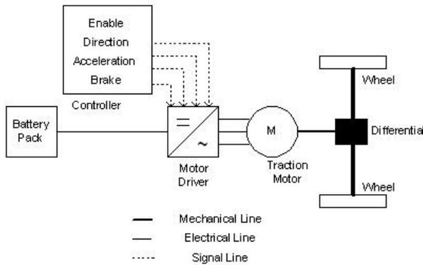
Fig. 15. EM electrical and mechanical connections
