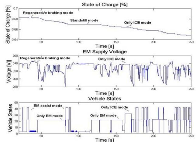
Fig. 17. Experimental result illustrating regenerative braking
