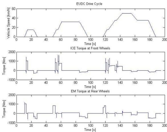
Fig. 10. EM and ICE torques during EUDC at wheels
