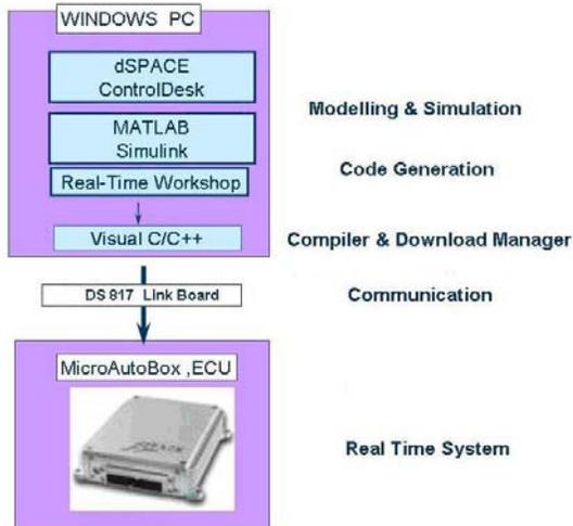
Fig. 14. Rapid HEV control algorithm prototyping process diagram
