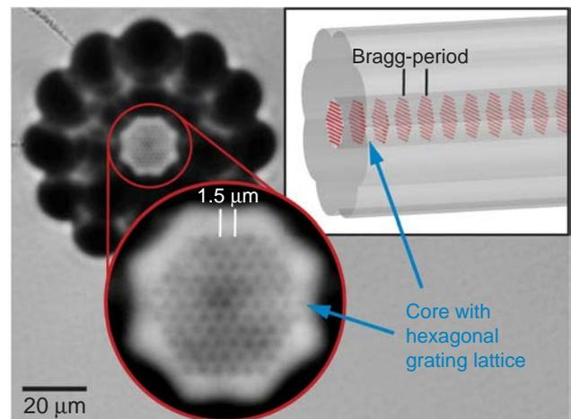
Fig. 1. (Color online) End-on, brightfield microscope image of the WBG revealing the hexagonal lattice of point features within the core of the waveguide. The inset shows a three-dimensional rendering of the structure (not to scale).
