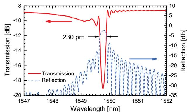
Fig. 3. (Color online) Transmission and reflection spectrum of a 5.8 mm long DCWBG showing a 10.5 dB transmission dip and a 230 pm (3 dB) wide reflection peak with a coupling constant  $\kappa L = 1.88$ .
