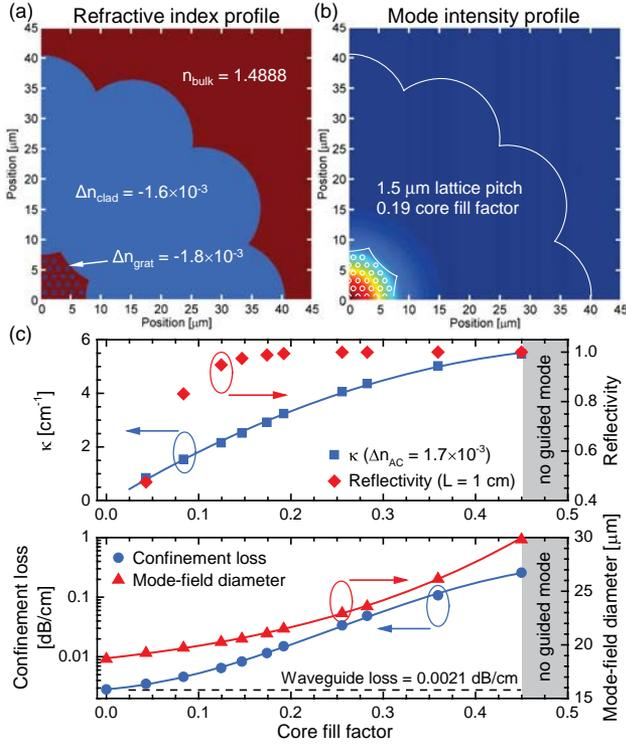
Fig. 4. (Color online) (a) Example of a refractive index profile with 1.5  $\mu\text{m}$  pitch grating (0.19 core fill factor) used for modeling. (b) Corresponding guided mode intensity profile. (c) Coupling constant  $\kappa$ , grating reflectivity, CL and MFDs of the guided mode versus the fill factor. The solid lines are a guide for the eye only.
