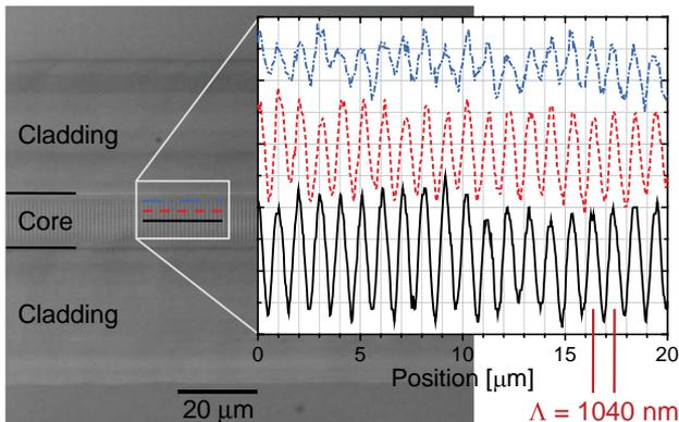
Fig. 2. (Color online) Top-down differential interference contrast image of the WBG with line profiles of the grating at three different positions showing the grating phase relation across the core. A reduction of grating contrast is apparent in close proximity to the cladding (top profile).
