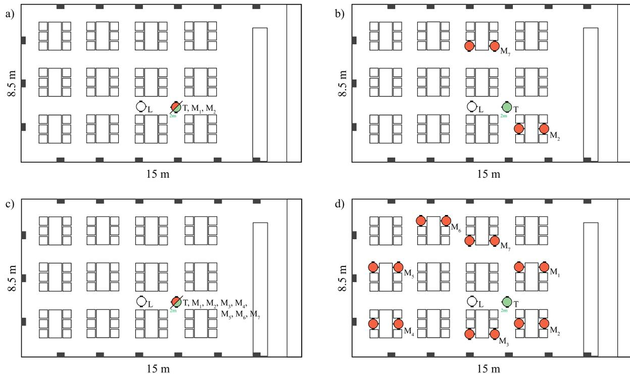
FIG. 2. (Color online) Top-down view of cafeteria simulated in ODEON. The listener position ( $L$ ) faces the target ( $T$ ) at 2 m distance. The two-talker maskers (with each dialogue denoted as  $M_1 - M_7$ ) were either distributed in the room or colocated with the target ( $T$ ).
