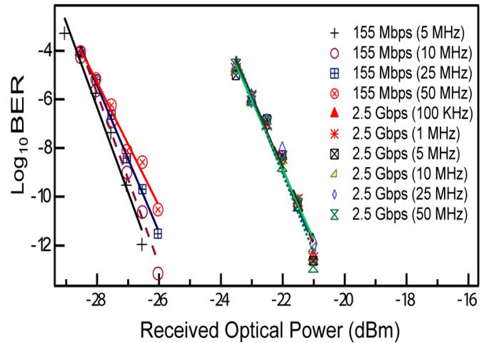
Figure 4. BER for different laser linewidths and data rates
