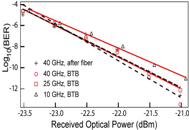
Figure 2. BER curves for different frequency spacing between two lasers
