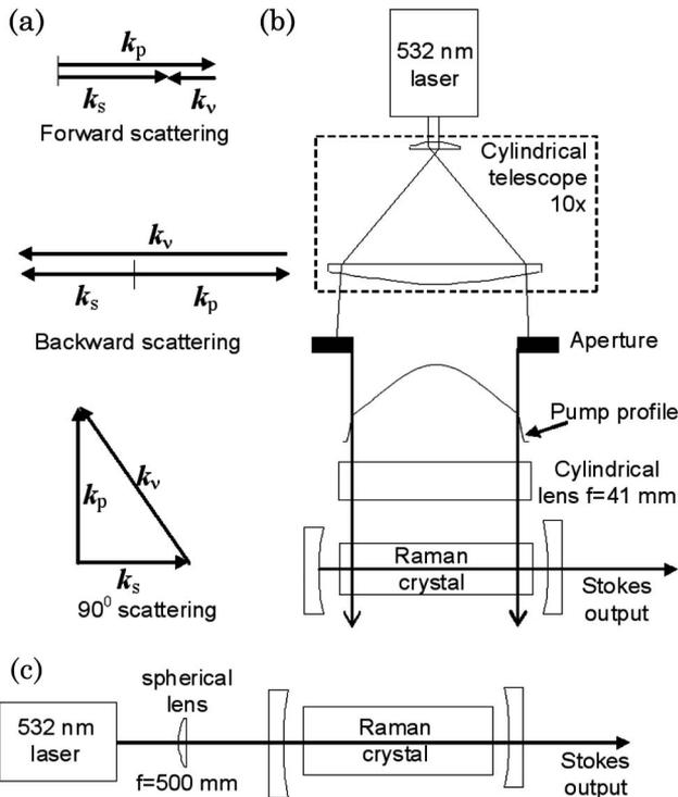
Fig. 1. (a) Phase-matching diagrams showing the range of  $k_\nu$  vector magnitudes and directions for forward, backward, and  $90^\circ$  scattering. Schematic of the (b) side-pumped and (c) end-pumped Raman lasers.
