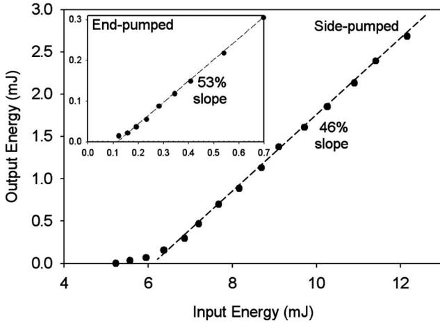
Fig. 2. Output energy as a function of the pump energy transmitted by the pump face of the crystal for the side-pumped and end-pumped (inset) configurations.
