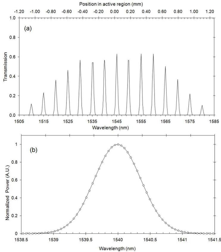
Fig. 3. (a) Total IPS efficiency across the full laser wavelength tuning range (this corresponds to  $\sim$ 90% of the device active area). Each peak corresponds to a series of focal plane measurements at a fixed input laser wavelength. (b) High-resolution de-convolved measurement of the output IPS spectral point spread function obtained by tuning the central laser wavelength by 0.05nm increments at a fixed fiber position in the focal plane.
