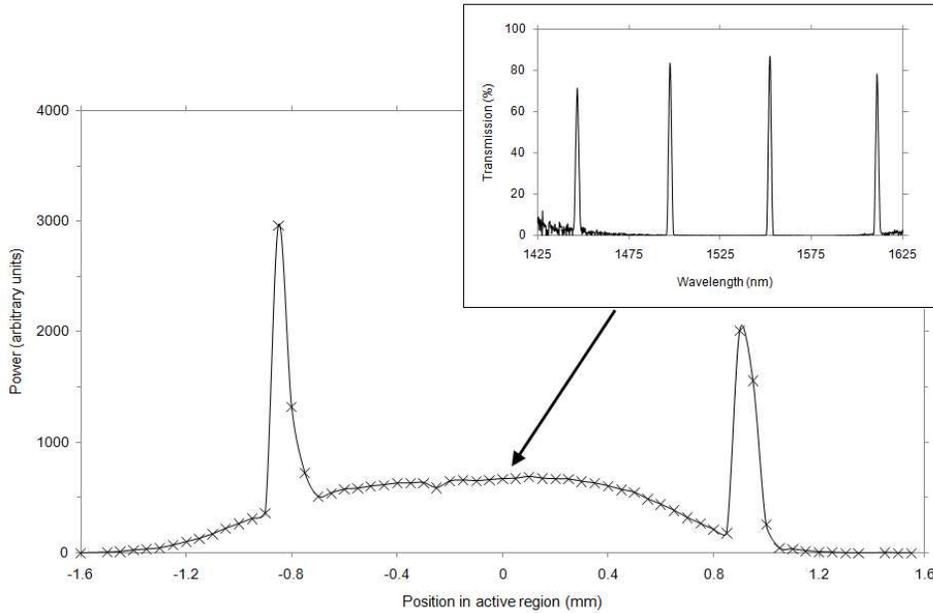
Fig. 4. Power output across the full IPS focal plane (measured by translating a fiber) with the input laser locked to  $1580\text{nm}$ . The two peaks are adjacent orders of the same laser wavelength. Insert: Normalized spectral measurement (using the OSA) with the fiber fixed in the IPS focal plane position indicated by the arrow, demonstrating the transmission of higher diffraction orders from the wings of the laser gain profile.
