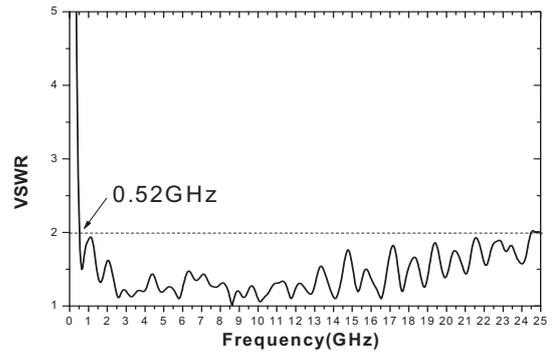
Fig. 2 VSWR of proposed antenna ( $d=4.2\text{mm}$ )
