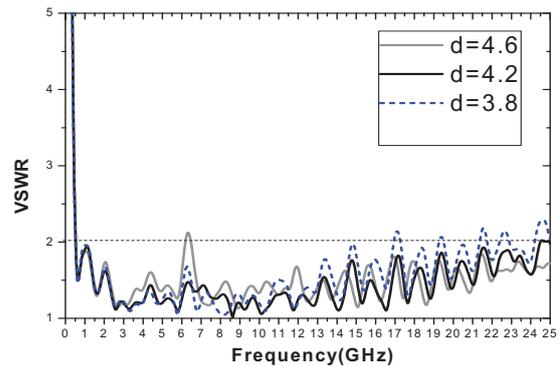
Fig. 4 The VSWR of the antenna with different radius  $d$
