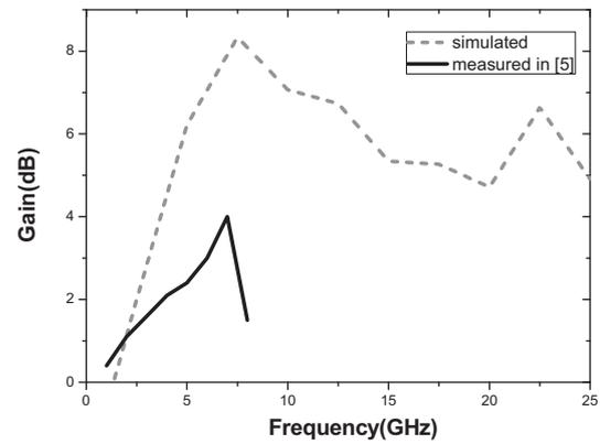
Fig. 7 Comparison between simulated gain of proposed antenna and measured gain of [5]
