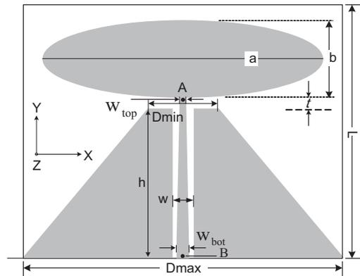
Fig. 1 (a) A standard elliptical printed monopole antenna fed by a tapered CPW line
