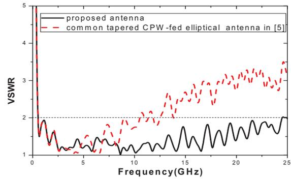
Fig. 3 VSWR comparison between the proposed antenna and the common tapered CPW-fed elliptical monopole antenna in [5]
