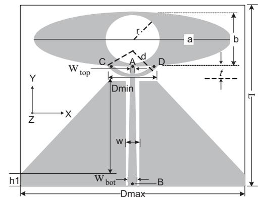
Fig. 1 (b) The proposed antenna ( $D_{max}=124$  mm,  $L=90$ mm,  $D_{min}=9$ mm,  $a=120$ mm,  $b=30$ mm,  $t=2.3$  mm,  $r=14$ mm,  $w_{top}=1$ mm,  $w_{bot}=2.6$ mm,  $w=3$ mm,  $t=2.3$ mm,  $h1=5$ mm,  $h=50$ mm,  $d=4.2$ mm)
