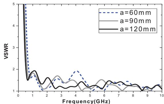
Fig. 5 The VSWR of the antenna with different major axis  $a$  of the elliptical patch
