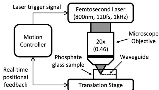
Fig. 1. Experimental setup for multiwavelength WGL fabrication.
