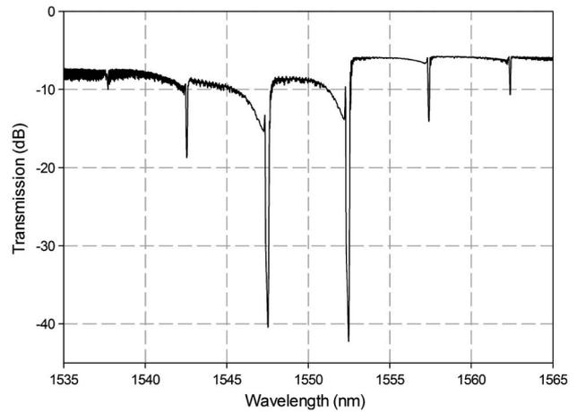
Fig. 4. Transmission spectrum of a  $\pi/2$  phase-modulated sampled WBG fabricated in Yb-doped phosphate glass. The central Bragg resonance is suppressed while odd harmonic sideband resonances emerge. This complex grating structure was written in a single fabrication step without any postprocessing.
