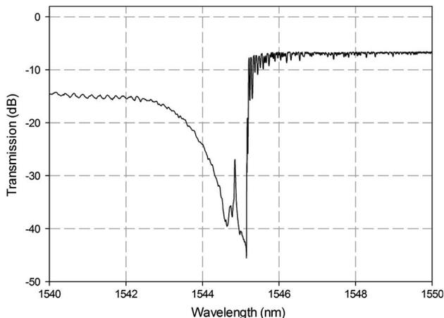
Fig. 3. Transmission spectrum of a 20 mm long WBG in Yb-doped phosphate glass with a  $\pi/2$  phase shift spatially located in its center. The gradual decrease in transmission up to the Bragg resonance is indicative of the radiation modes of the grating in a geometry that has no well-defined cladding.
