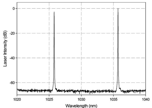
Fig. 5. Output spectrum, at full pump power, of a dual-wavelength laser fabricated in a 10 nm long Yb-doped phosphate glass using a  $\pi/2$  phase-modulated sampled DFB WBG. The ordinate axis scale is referenced to the peak.
