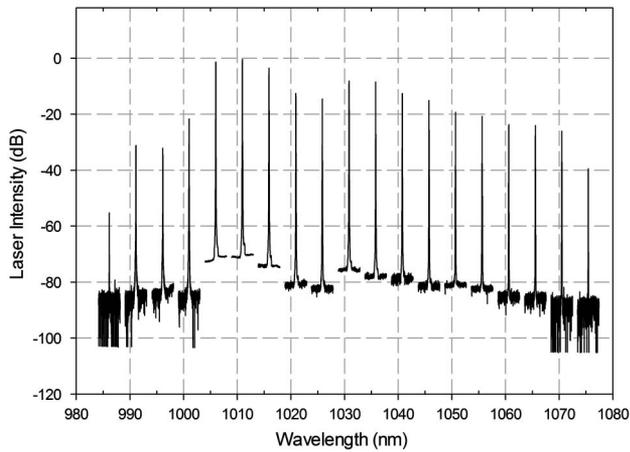
Fig. 2. Output spectra of multiple 10 nm long WGLs plotted on the same axes demonstrating a gain bandwidth of approximately 100 nm.
