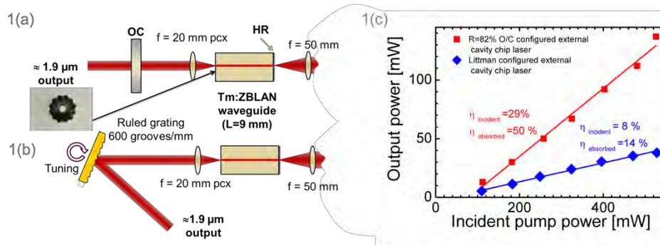
Fig. 1. (a):  $\text{Tm}$ :ZBLAN waveguide laser configured for external cavity operation using an output coupler mirror. Figure 1(b). A Littrow configured external cavity containing a diffraction grating. Inset: A microscope end view of the depressed cladding waveguide. Figure 1c. Measured slope efficiency for the Ti:sapphire pumped external cavity  $\text{Tm}$ :ZBLAN laser and Littrow configured external cavity laser.
