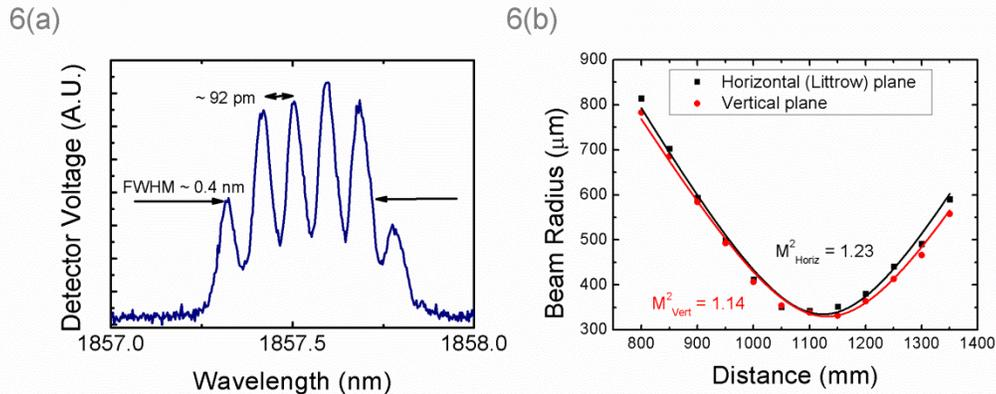
Fig. 6. (a). Time-averaged spectrum of the tuned output of the Littrow configured extended cavity chip laser. Fig. 6(b). Measured beam quality ( $M^2$ ) of the Littrow configured extended cavity chip laser.
