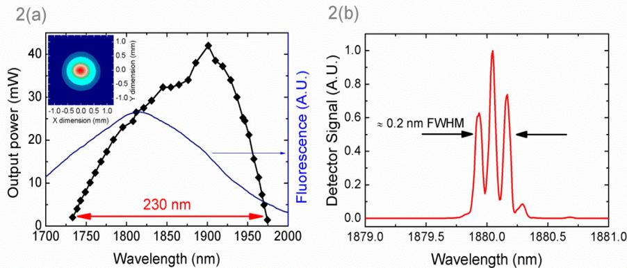
Fig. 2. (a). Measured tuning range of the Tm:ZBLAN chip with the thulium fluorescence spectrum overlaid. Fig. 2(b). A typical lineshape of the Littrow configured cavity. The fringes correspond to the  $L = 9$  mm waveguide chip acting as a Fabry-Pérot etalon.
