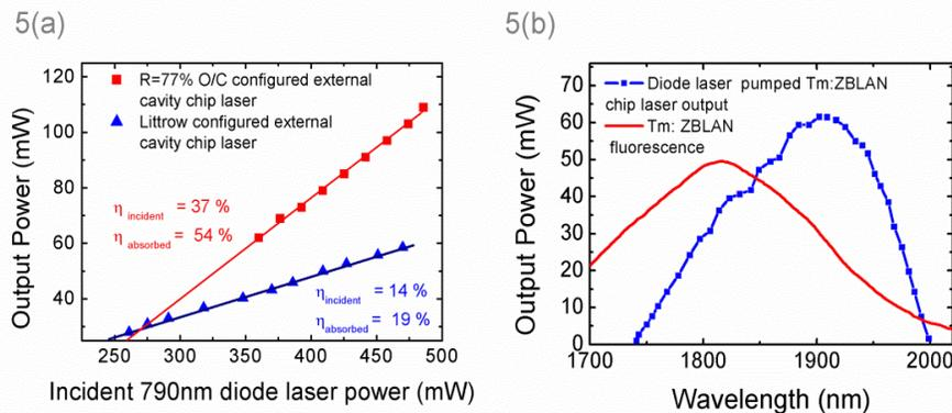
Fig. 5. (a). Slope efficiencies of the laser diode pumped  $L = 12$  mm Tm: ZBLAN waveguide laser configured for external operation using either a  $R = 77\%$  OC or a 600 lines/mm diffraction grating. Fig. 5(b). Measured tuning range of the Littrow configured Tm:ZBLAN laser for an incident pump power of 475 mW. For reference the fluorescence emission of Tm:ZBLAN is overlaid.
