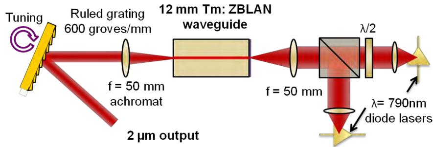
Fig. 4. Schematic of the twin 790nm diode-laser pumped Tm:ZBLAN waveguide laser.
