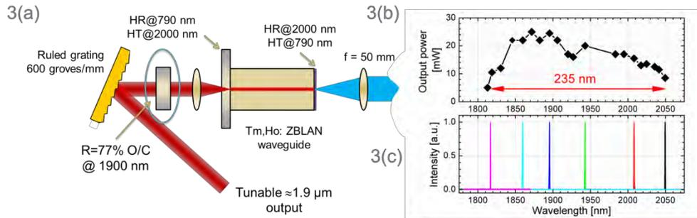
Fig. 3. (a). Modified Littrow external cavity Tm,Ho:ZBLAN waveguide laser using a R = 77% OC intra-cavity for additional cavity feedback. Fig. 3(b). Tuning curve for the Tm,Ho:ZBLAN waveguide laser. Fig. 3(c). Representative spectra across the tuning curve.
