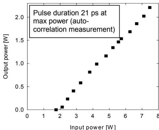
The maximum output power was 2.21 W. The laser threshold was approximately 2 W, leading to a slope efficiency of 41% and an absolute efficiency of 29%. The conversion efficiency is slightly higher than that obtained for potassium gadolinium tungstate (25.6%) [6], and our model suggests higher efficiencies are likely to be obtained with optimized resonator mirrors. The position of the output coupler is crucial to gaining efficient output and also strongly affects the output pulse duration.
