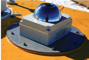
Figure 1. HRCAM installed on the roof of the PLATO instrument module at Dome A in 2010.
