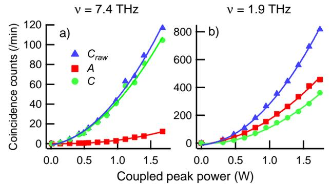
Fig. 3. (Color online) (a) Coincidence count rate versus peak power, for pairs generated in the low Raman window at  $\nu = 7.4$  THz. Here, the true coincidence count rate  $C$  approaches the total coincidence rate  $C_{\text{raw}}$ , as SFWM is dominant over noise  $A$ . (b) For small detuning  $\nu = 1.9$  THz,  $C$  and  $A$  are comparable, as SpRS is significantly more efficient at this detuning. Poissonian error bars are equal to the size of plot markers.
