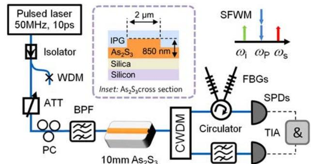
Fig. 1. (Color online) Experimental setup for correlated photon-pair generation via SFWM. ATT, attenuator; PC, polarization controller; SPD, single-photon detector; TIA, time interval analyzer; remaining acronyms defined in text. Inset: cross section of  $\text{As}_2\text{S}_3$  waveguide. IPG, inorganic polymer glass.
