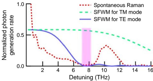
Fig. 2. (Color online) Calculation of the normalized photon generation rates versus detuning from the pump for  $\gamma P_0 L = 0.1$ . The short dashed line shows the SpRS rate [14], with a characteristic minimum at 7.4 THz (shaded). The long dashed and solid lines are the SFWM correlated pair generation for TM and TE modes, respectively. Pair generation extends to the low Raman window only for the TM mode [13].
