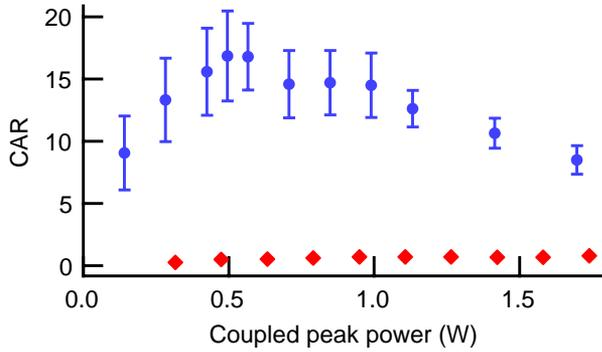
Fig. 4. (Color online) Measured CAR: for small detuning (red diamonds) and operating in the low Raman window (blue circles) with Poissonian errors bars included.
