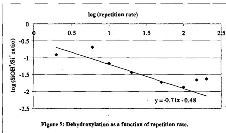
Figure 5: Dehydroxylation as a function of repetition rate.
