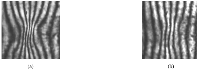
Fig. 4. Fringes (a) with and (b) without lasing at 8 W of absorbed power
