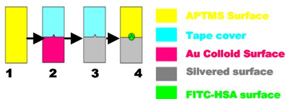
Figure 1. Schematic illustration of the deposition procedure for Au-core Ag-shell nanoparticles on glass surface (Top view). (1) APTMS modified glass surface; (2) Zero residual tape patterning and Au colloid deposition; (3) Silver enhancing deposition; (4) Patterning the interface with Press-to-seal silicone insulator; incubation with FITC-HSA.
