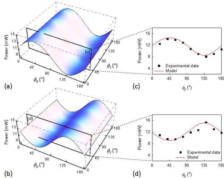
Fig. 1. Modeled (a)  $x$ - and (b)  $y$ -polarized output powers of a dual-polarization Nd:YAG laser pumped at  $1.2 \times$  threshold as a function of crystal angle ( $\phi_c$ ) and relative pump angle ( $\phi_p$ ). Corresponding experimental (c)  $x$ - and (d)  $y$ -polarized output powers as a function of pump polarization angle at a fixed crystal angle.
