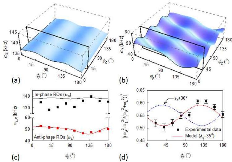
Fig. 3. Modeled (a) in-phase and (b) anti-phase RO frequency for a dual-polarization Nd:YAG laser pumped near threshold as a function of crystal angle ( $\phi_c$ ) and relative pump angle ( $\phi_p$ ). Corresponding (c) experimental in- and anti-phase RO frequencies and (d) Mode-coupling constant ( $C = [(\omega_R^2 - \omega_L^2) / (\omega_R^2 + \omega_L^2)]^2$ ) as a function of pump polarization angle.
