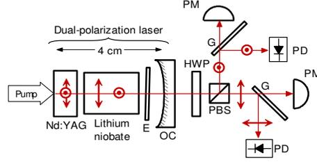
Fig. 2. Measurement arrangement of the polarized outputs (see Fig. 1) and polarization dynamics (see Fig. 3) of the dual-polarization laser.  $E$  is an etalon; OC laser output mirror; HWP is a half-waveplate; PBS is a polarization beam splitter; G are glass slides reflecting ~4%; PM are optical power meters; and PD are >1 MHz bandwidth photodiodes.
