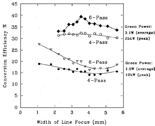
Fig. 6. Variation in peak conversion efficiencies (four-pass and six-pass, based on green depletion), with the width of the focused beam and for two different pump power levels (3.1 W average, and 1.0 W average).
