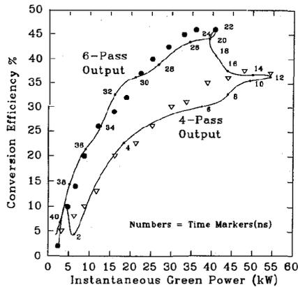
Fig. 4. Instantaneous green SHG conversion efficiency as a function of instantaneous pump intensity derived from the pump and depleted pump pulse shapes. Times (in ns) during the pump pulse are indicated by small numbers along the curve. Points derived from peak conversions of the four-pass and six-pass outputs given in Fig. 3 are also plotted for comparison.
