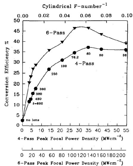
Fig. 5. Variation in peak conversion efficiencies (four-pass and six-pass, based on green depletion), with the focal length of the cylindrical lens. Conversion efficiency is plotted as a function of  $1/F$ -number, and also the resulting peak focal power densities for the four-pass and six-pass outputs. The actual focal lengths of the cylindrical lenses used are also indicated. Note the beam width was 3.75 mm.
