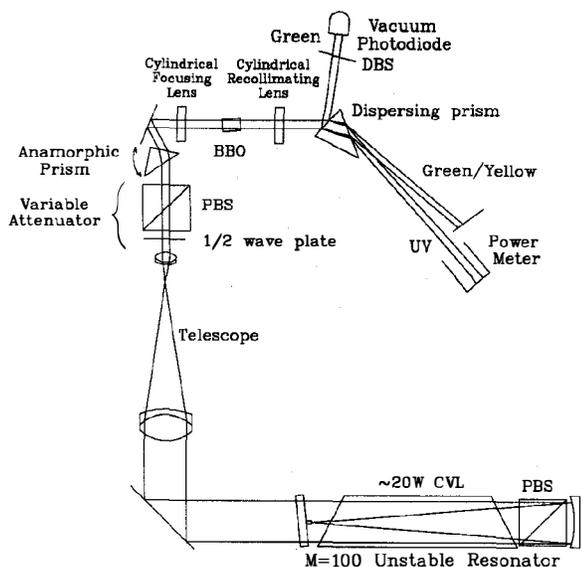
Fig. 1. Experimental layout for second-harmonic and sum-frequency generation of the CVL.
