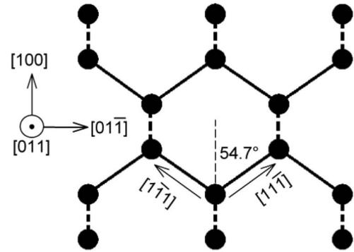
Fig. 2. Diamond crystal lattice as viewed along the direction of laser propagation. Dashed lines represent bonds not contained within a plane parallel to the page.
