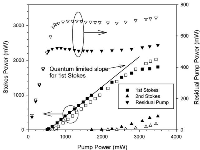
Fig. 3. Stokes powers and residual pump power for increasing pump input. Filled markers are for pump polarization aligned with [111]. Hollow markers are for pump aligned with [100].
