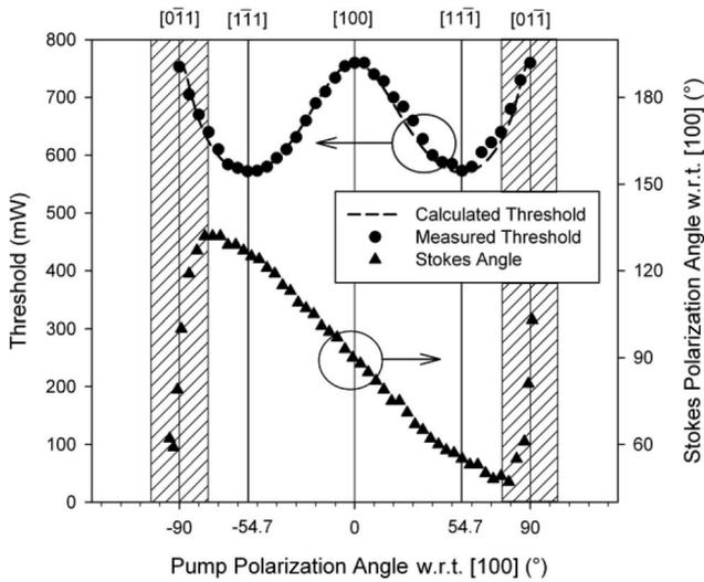
Fig. 1. First Stokes threshold and polarization angle for varying pump polarization angle. The shaded regions represent areas where two orthogonal polarizations are above threshold for 1.4 W of pump.
