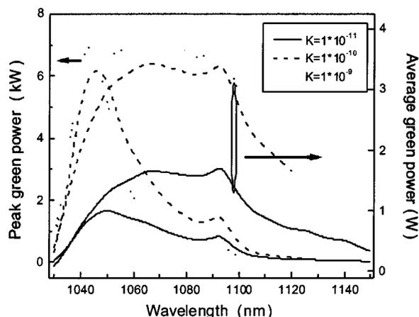
Fig. 8. Calculated peak and average green powers as a function of emission wavelength for several nonlinear coupling coefficients. (Calculated in a high- $Q$  cavity at 10 kHz, taking into account emission cross section and lower-level fractional population).
