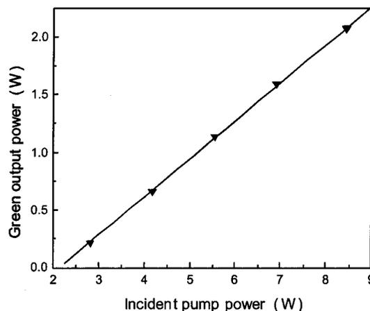
Fig. 4. Measured average green power as a function of incident pump power (including a linear fit), by use of a high- $Q$  cavity.
