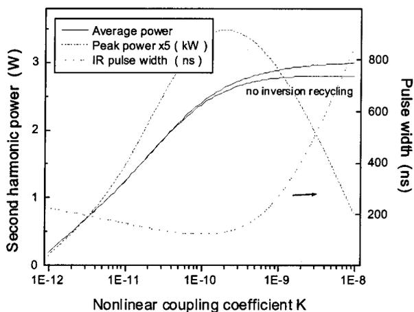
Fig. 6. Numerical calculation for average and peak green powers and infrared pulse width (FWHM) as a function of nonlinear coupling coefficient.
