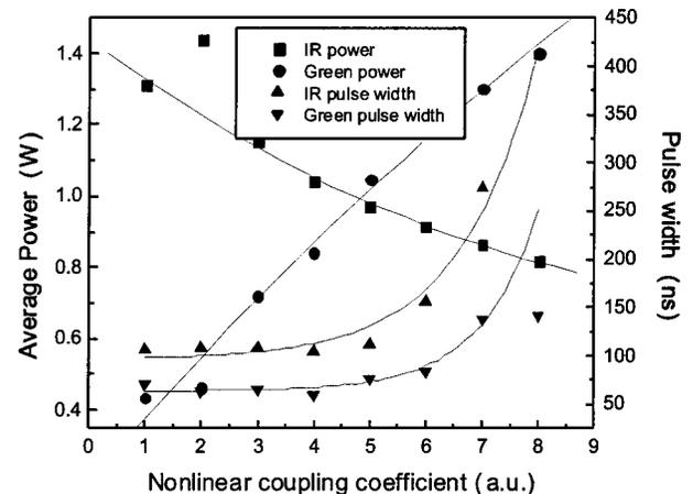
Fig. 2. Measured infrared and green average powers and pulse widths as a function of phase mismatch (higher numbers correspond to higher nonlinear coupling coefficients). Solid curves are drawn to guide the eye, 99.5% reflectivity output coupler; prf = 10 kHz
