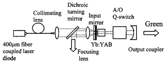
Fig. 1. Experimental setup for end-pumped  $Q$ -switched operation in Yb:YAB.
