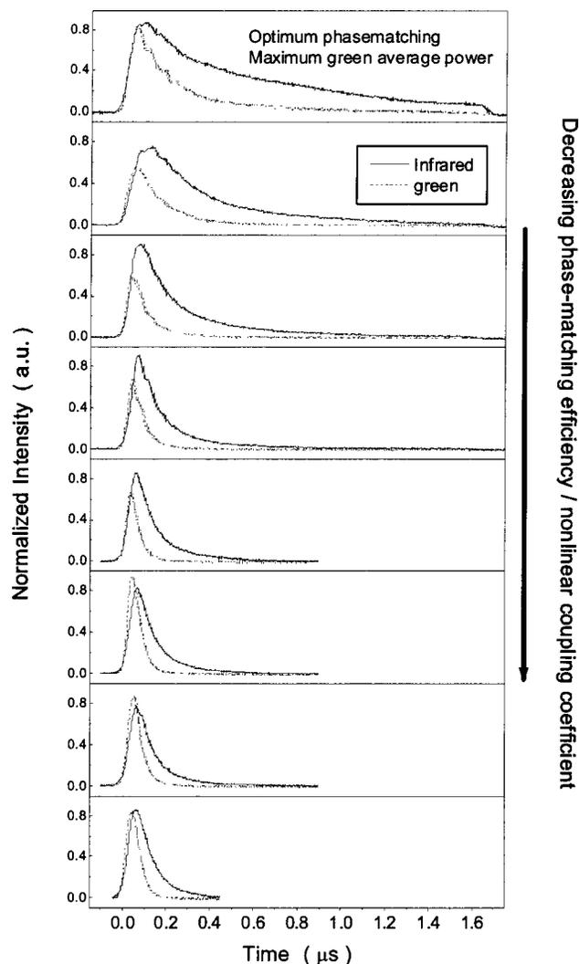
Fig. 3. Normalized infrared and green temporal outputs as a function of phase mismatch, (nonlinear coupling coefficient). (99.5% reflectivity output coupler; prf = 10 kHz).
