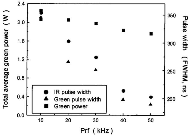
Fig. 5. Measured average green power and infrared and green pulse width as a function of pulse repetition frequency at maximum pump power (8.5 W) in a high- $Q$  cavity.
