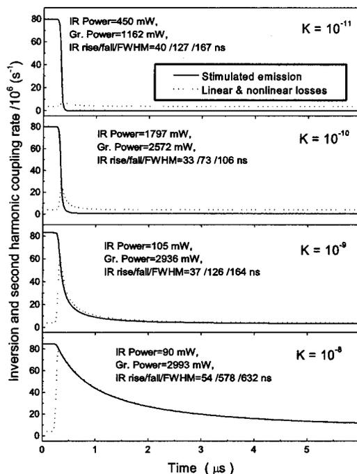
Fig. 7. Calculated stimulated emission rate and total loss (linear and nonlinear) rate as a function of time for different nonlinear coupling coefficients ( $K$ ).
