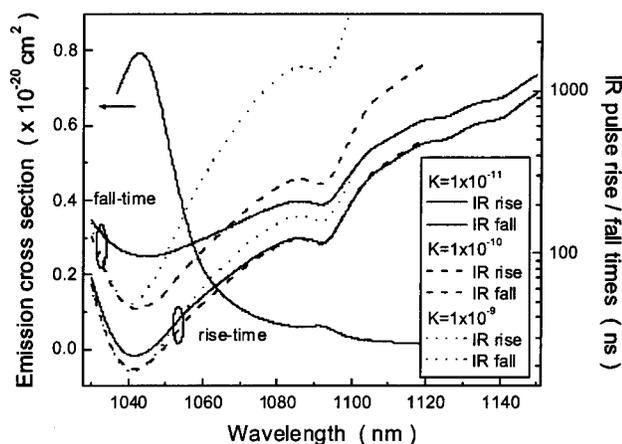
Fig. 9. Calculated infrared pulse rise and fall times (for several nonlinear coupling coefficients) and measured emission cross section as a function of wavelength. (Rise and fall times calculated in a high- $Q$  cavity at 10 kHz, taking into account emission cross section and lower-level fractional population).
