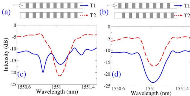
Fig. 3. (Color online) Experimental results. Coupler geometry: (a) symmetric and (b) antisymmetric. Measured transmission spectra from the first (solid) and the second (dashed) waveguides of (c) symmetric and (d) antisymmetric coupler when the light is coupled to the first waveguide.
