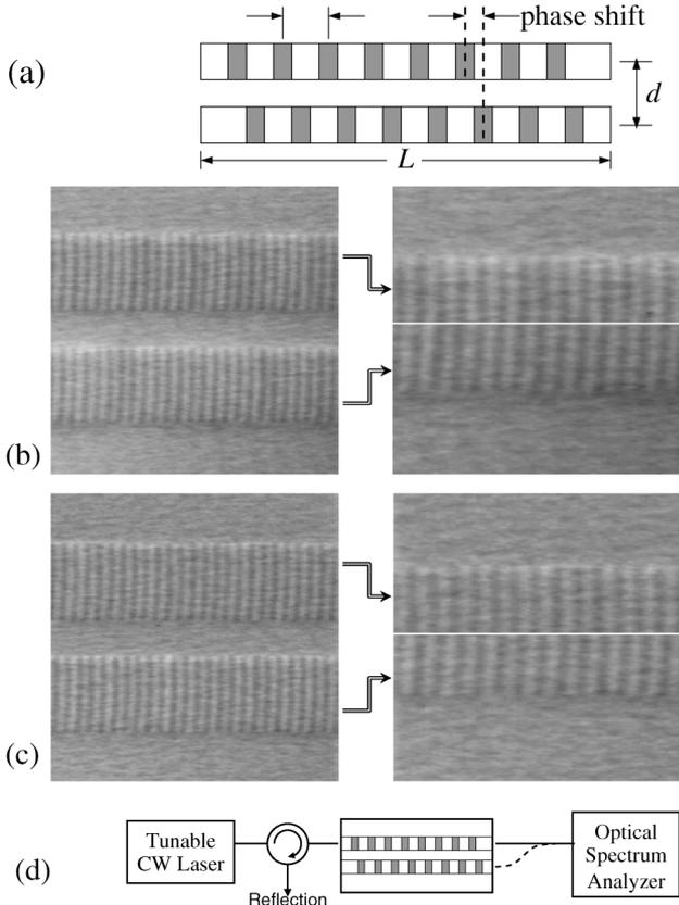
Fig. 1. (a) Schematic of the Bragg grating coupler. Transmission differential interference contrast micrographs of (b) symmetric and (c) antisymmetric Bragg couplers. The 500 nm grating pitch is clearly visible in the horizontal direction while the vertical scale has been compressed by a factor of 4 for clarity. (d) Bragg grating coupler characterization setup.
