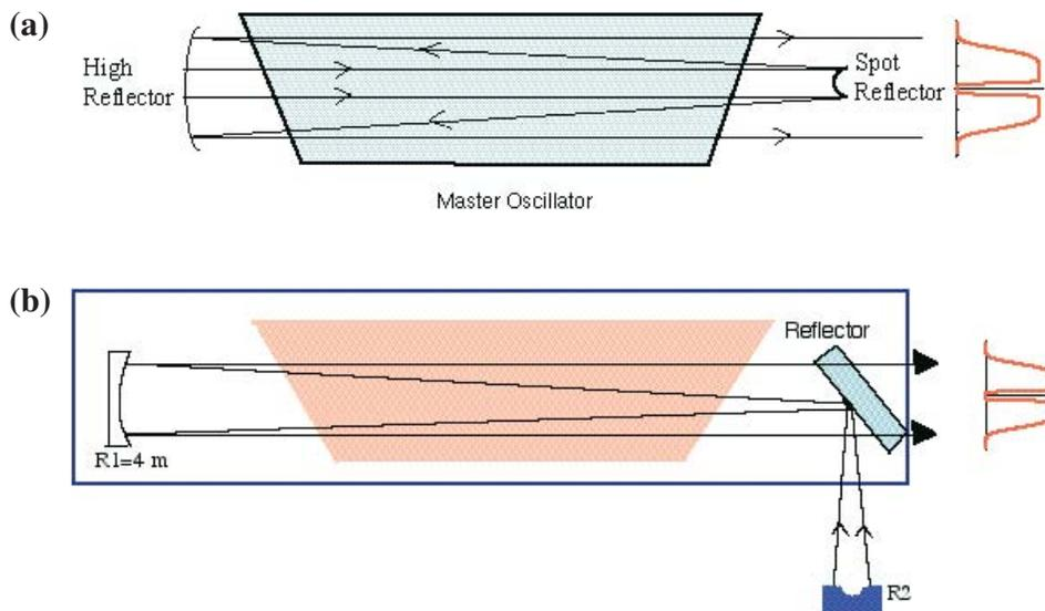
**Fig. 2.** Characteristic intensity modulations corresponding to round-trip time in the resonator of a copper vapour laser.
