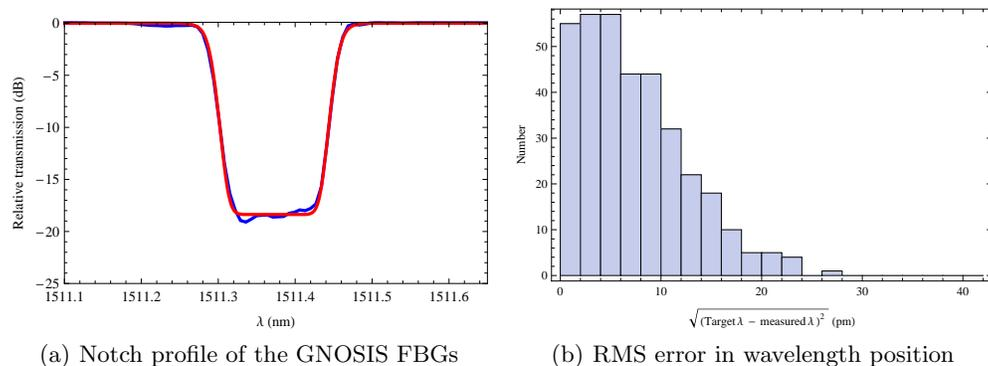
**Figure 2.** The properties of the GNOSIS FBGs. The notch profiles (a) are very square, narrow and deep, allowing efficient filtering of the OH lines. The blue lines shows a measured profile and the red line shows the best fitting Butterworth function. The notch wavelengths measured from 8 different FBGs are accurate to an RMS error of 11 pm. The accuracy of all notches to within < 30 pm will ensure that the OH lines are suppressed by the 200 pm wide notch.
