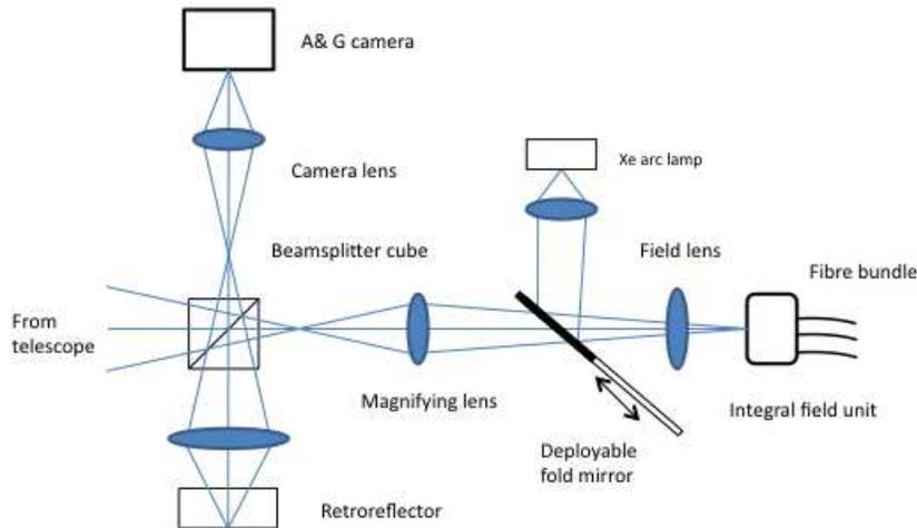
**Figure 3.** Schematic diagram of the GNOSIS fore-optics.
