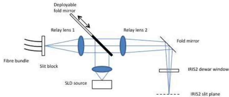
**Figure 4.** Schematic diagram of the GNOSIS relay optics.
