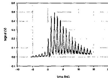
Fig. 2 Temporal profile of first Stokes output
