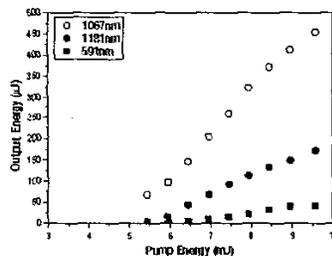
Fig.1 Output energy vs pump diode energy.
