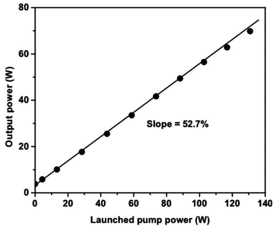
Fig. 2. Slope efficiency of the amplifier stage.
