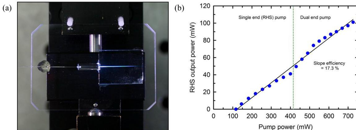
Fig. 1. (a) A pigtailed waveguide oscillator device operating at 1.032  $\mu\text{m}$  fabricated in Ytterbium-doped phosphate glass using the femtosecond laser direct-write technique and its (b) laser output power as a function of pump power for single and dual end pump geometries.
