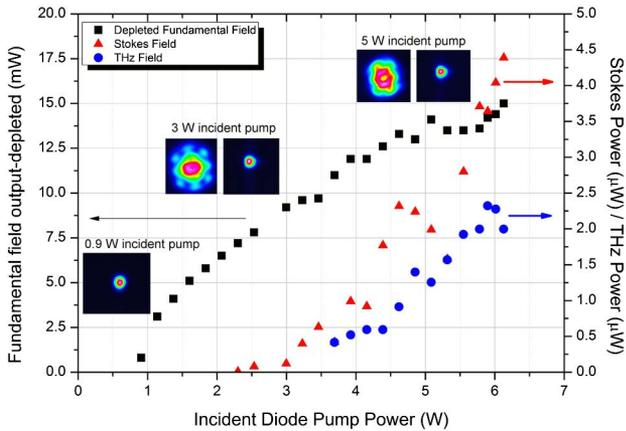
Fig. 2. Power scaling properties of the depleted fundamental, Stokes and THz fields, with the Stokes resonator angled to generate 1.83 THz emission. Shown inset are mode profiles of the fundamental (left) and Stokes (right) fields at incident pump powers of 0.9 W, 3 W and 5 W; note that the Stokes field is not present for an incident pump power of 0.9 W (below SPS threshold).
