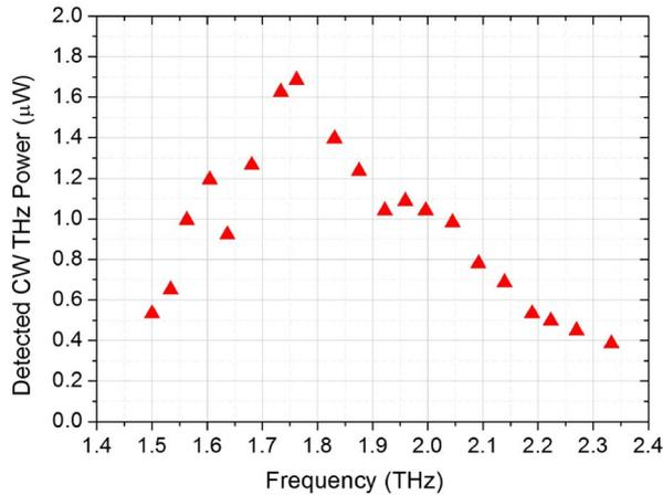
Fig. 3. Change in detected THz power as a function of THz field frequency. Input pump power was set to 5.2 W.
