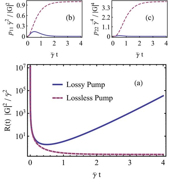
FIG. 7. (Color online) (a) Plot of the dimensionless  $R(t)|G|^2/\bar{\gamma}^2$  in two cases: dashed (red) curve, when  $\gamma_p = 0$ ; and solid (blue) curve, when  $\bar{\gamma} = \gamma_p$ . (b, c)  $p_{11}$  and  $p_{22}$  as a function of time for the same conditions.
