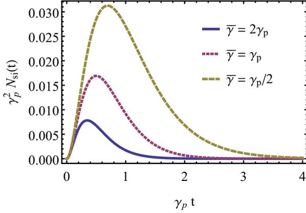
FIG. 2. (Color online) Dimensionless two-photon expectation in three cases: dashed (green) curve, when  $\bar{\gamma} = \gamma_p/2$ ; dotted (red) curve, when  $\bar{\gamma} = \gamma_p$ ; and solid (blue) curve, when  $\bar{\gamma} = 2\gamma_p$ .
