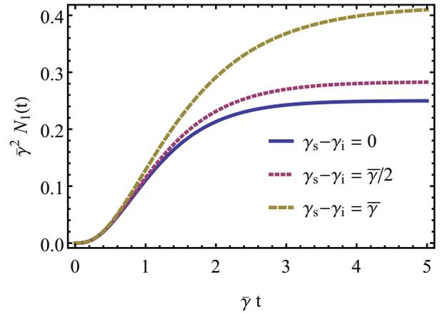
FIG. 5. (Color online) Dimensionless  $N_1(t)$  as a function of time in three cases: solid (blue) curve, when  $\gamma_s - \gamma_i = 0$ ; dotted (red) curve, when  $\gamma_s - \gamma_i = \bar{\gamma}/2$ ; and dashed (green) curve, when  $\gamma_s - \gamma_i = \bar{\gamma}$ .
