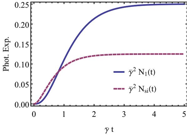
FIG. 4. (Color online) Photon dynamics when the pump mode is lossless but  $\gamma_s = \gamma_i$ . The two-photon expectation [dashed (red) curve] is compared to the one-photon-only expectation [solid (blue) curve]. Note that the plotted quantities are both dimensionless.
