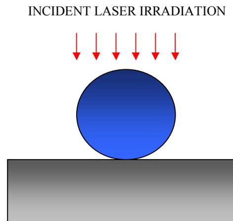
Figure 1: Microsphere-on-a-plane substrate subject to irradiation by a plane laser beam.
