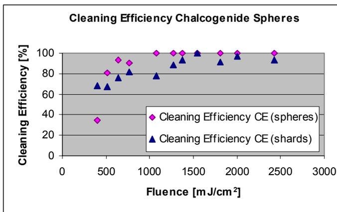
Figure 5: Cleaning Efficiency calculation for laser cleaning of chalcogenide spheres and shards from fused silica glass.
