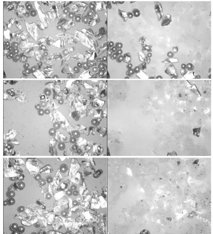
**Figure 4:** Before (left) and after (right) images of the laser cleaning experiments. Fluences for the images are top:  $399 \text{ mJ/cm}^2$ ; middle:  $1270 \text{ mJ/cm}^2$ ; bottom:  $2429 \text{ mJ/cm}^2$ . Image size is  $1.38 \times 1.04 \text{ mm}^2$ .
