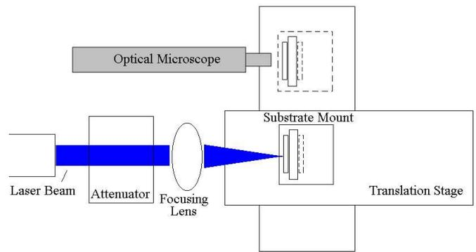
**Figure 3:** A schematic of the set-up used for the laser cleaning experiments.
