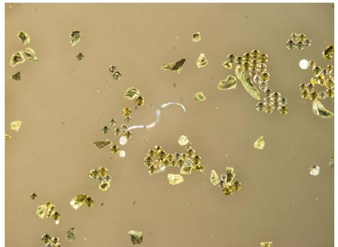
Figure 2: Image of chalcogenide spheres on a fused silica substrate imaged using a DIC optical microscope. Image size is 3.1 x 2.2 mm<sup>2</sup>.
