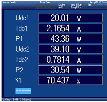
FIGURE 12 Experimental power profile of CPT system using WT1800 Precision Power Analyzer.
