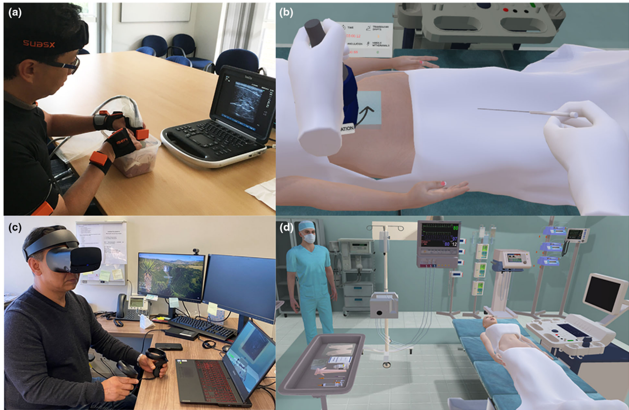
Figure 1 (a) Author AC wearing high-resolution motion capture hardware to create a video library of ultrasound images linked to spatial co-ordinates of a real-life ultrasound transducer. (b) The virtual reality software can use this database to faithfully display accurate imaging and needle position in response to movements of the virtual transducer and needle-holding hand. (c) Author AK demonstrating use of the virtual reality software. (d) Virtual reality simulation of operating theatre.
