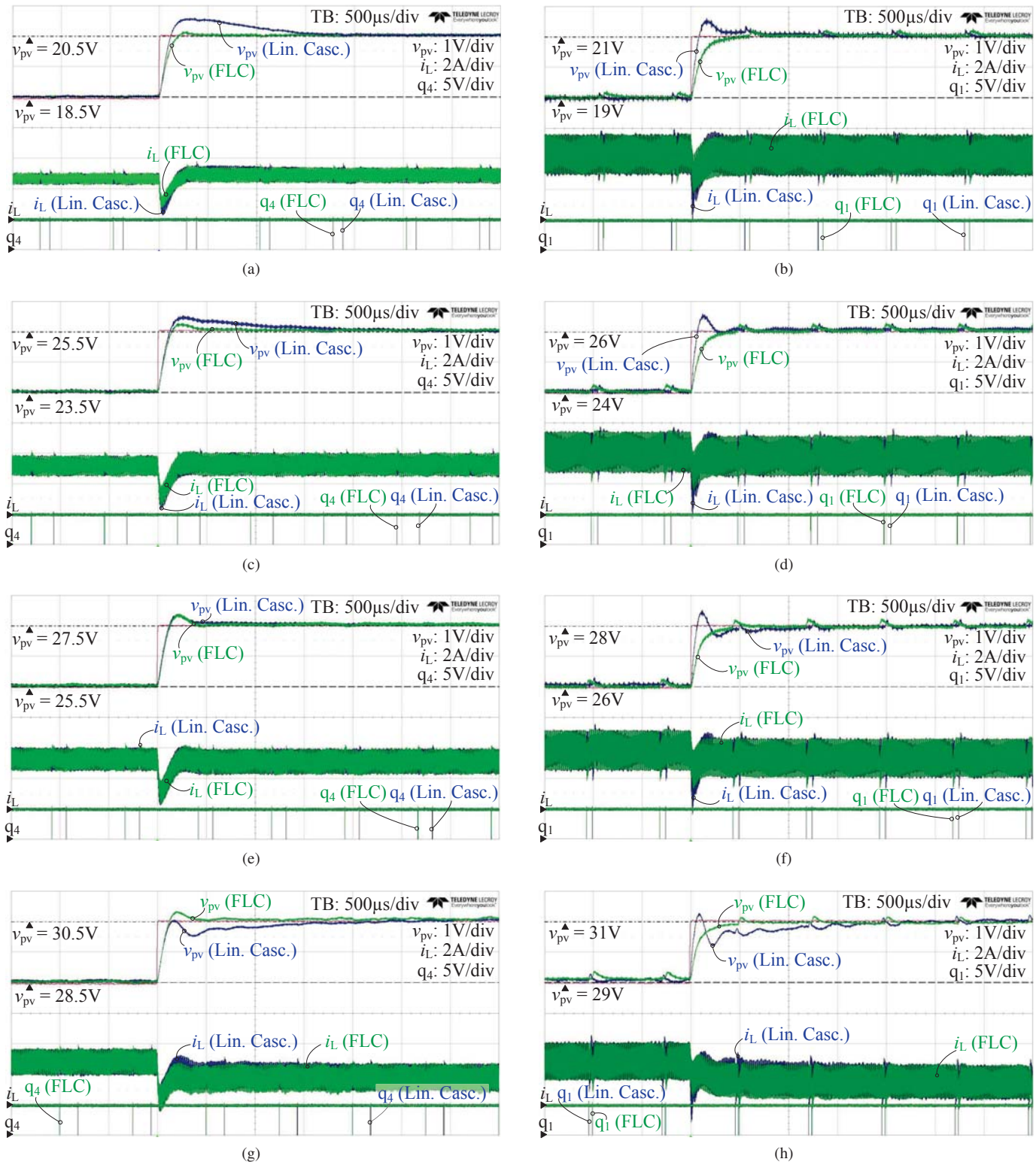
Fig. 13. PV voltage and inductor current behavior in response to PV voltage reference steps (green: FLC, blue: linear cascaded controller, pink: v_{pv}^* ). (a) Buck mode in the current source region (18.5-20.5V). (b) Boost mode in the current source region (19-21 V). (c) Buck mode in the MPP region (23.5-25.5 V). (d) Boost mode in the MPP region (24-26 V). (e) Buck mode in the MPP region (25.7-27.5 V). (f) Boost mode in the MPP region (26-28 V). (g) Buck mode in the voltage source region (28.5-30.5 V). (h) Boost mode in the voltage source region (29-31 V).
