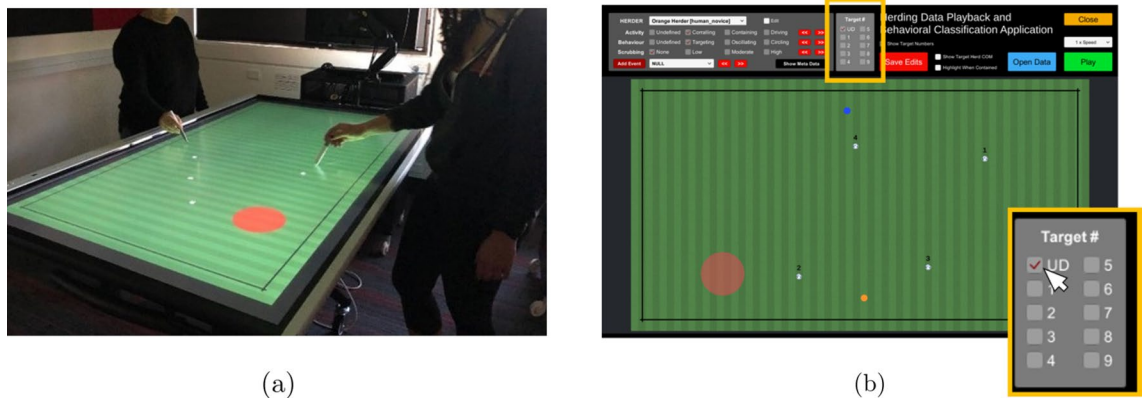
Figure 1. (a) The herding task and experimental setup. (b) A screenshot of the data playback and coding application used to identify which target a herder was corraling at each time step. The blue and orange dots are the herders and the white dots are the targets. The text label above each target specifies the target number (i.e., 1 to 4). The transparent red area is the containment region, which for the data employed here was always in the center of the game field. The insert panel on the bottom right of (b) is the target coding panel, where UD = no target. See main text for more details.
